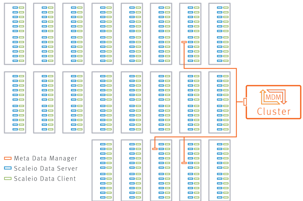
Figure 6 Physical layout example—3-node cluster
