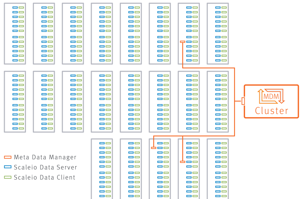
Figure 9 Physical layout example—3-node cluster
