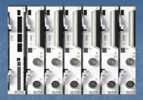
The radio shelf in RBS 6000 base stations supports a wide variety of RUs and DUs for all main frequency bands and any combination of Radio Frequency (RF) technologies (GSM, WCDMA, or LTE). Each radio shelf supports up to 6 RUs and a fully configured RBS6102 can house up to 12 RUs.
