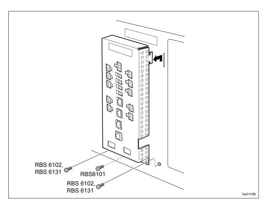
9. Push the SCU upwards and pull it towards the front of the cabinet to remove the SCU as shown in step 8 on page 3.
