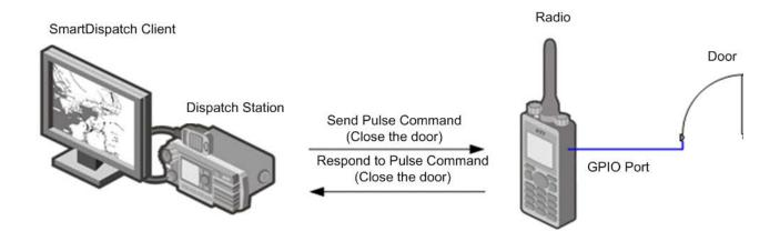
To apply the Telemetry feature, you should connect the monitored device to the GPIO port of the radio, define the telemetry commands (as below) and enable the radio in the following steps to respond the commands (see "7.5 Telemetry").
