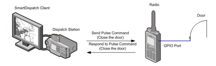
To apply the Telemetry feature, you should connect the monitored device to the GPIO port of the radio, define the telemetry commands (see "10.9 Telemetry") and enable the radio in the following steps to respond to the commands.
