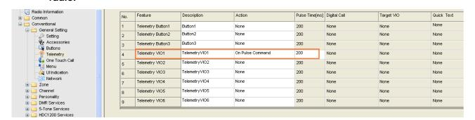
**Step 3** Set the GPIO port corresponding to the preset VIO port of the radio. The radio will respond to the telemetry command through this port.
