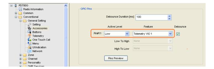
Different telemetry responses need different GPIO voltages. Here we take low level of the GPIO port as the active level.
