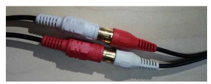
**Step 4** Plug the other end of the breakout cable into the speaker jack of the dispatch station. See the connection as follows.
