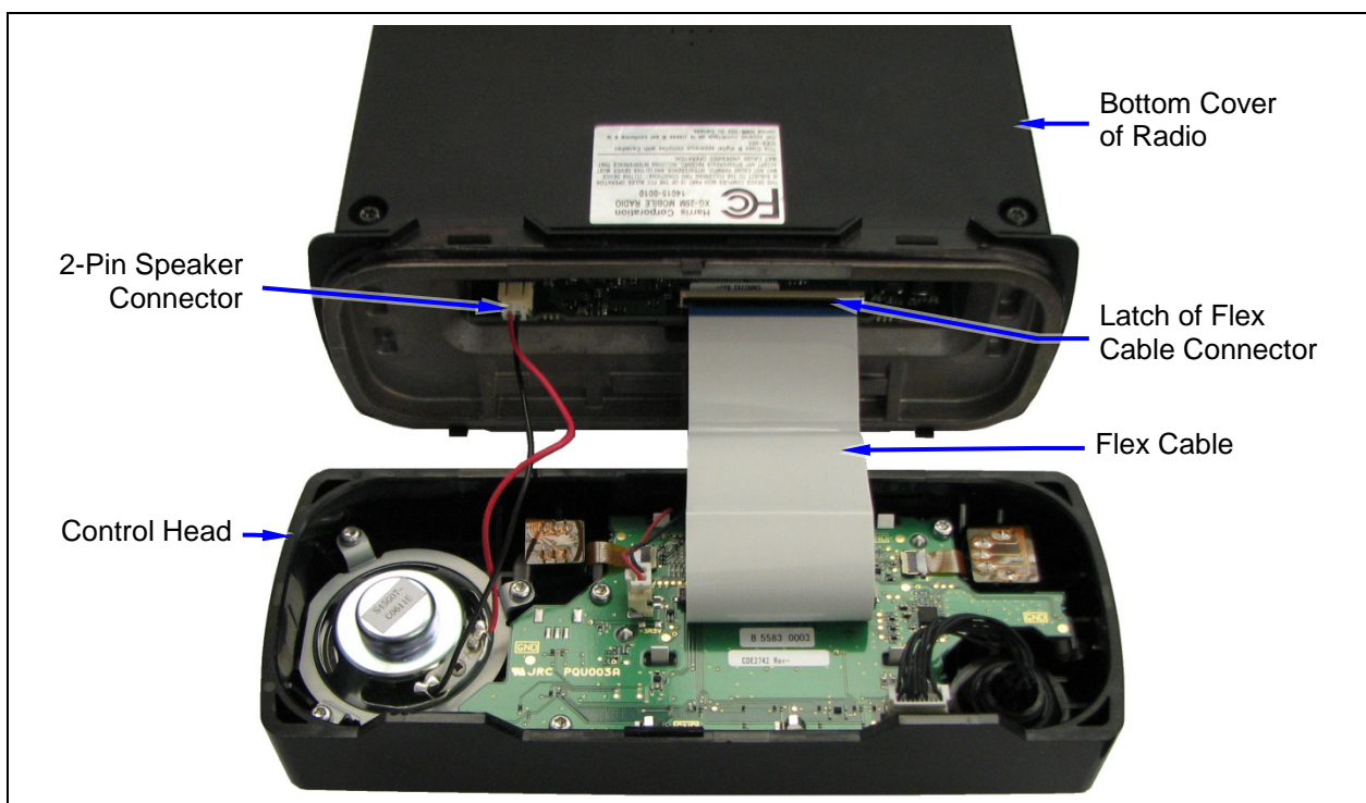
Figure 14-2: Removing the Control Head (2 of 2)
