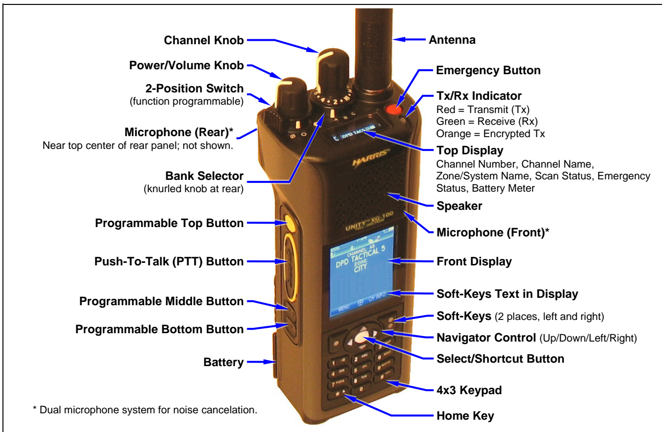
Figure 3-3: Unity XG-100P Portable Radio—Operating Controls and Displays
