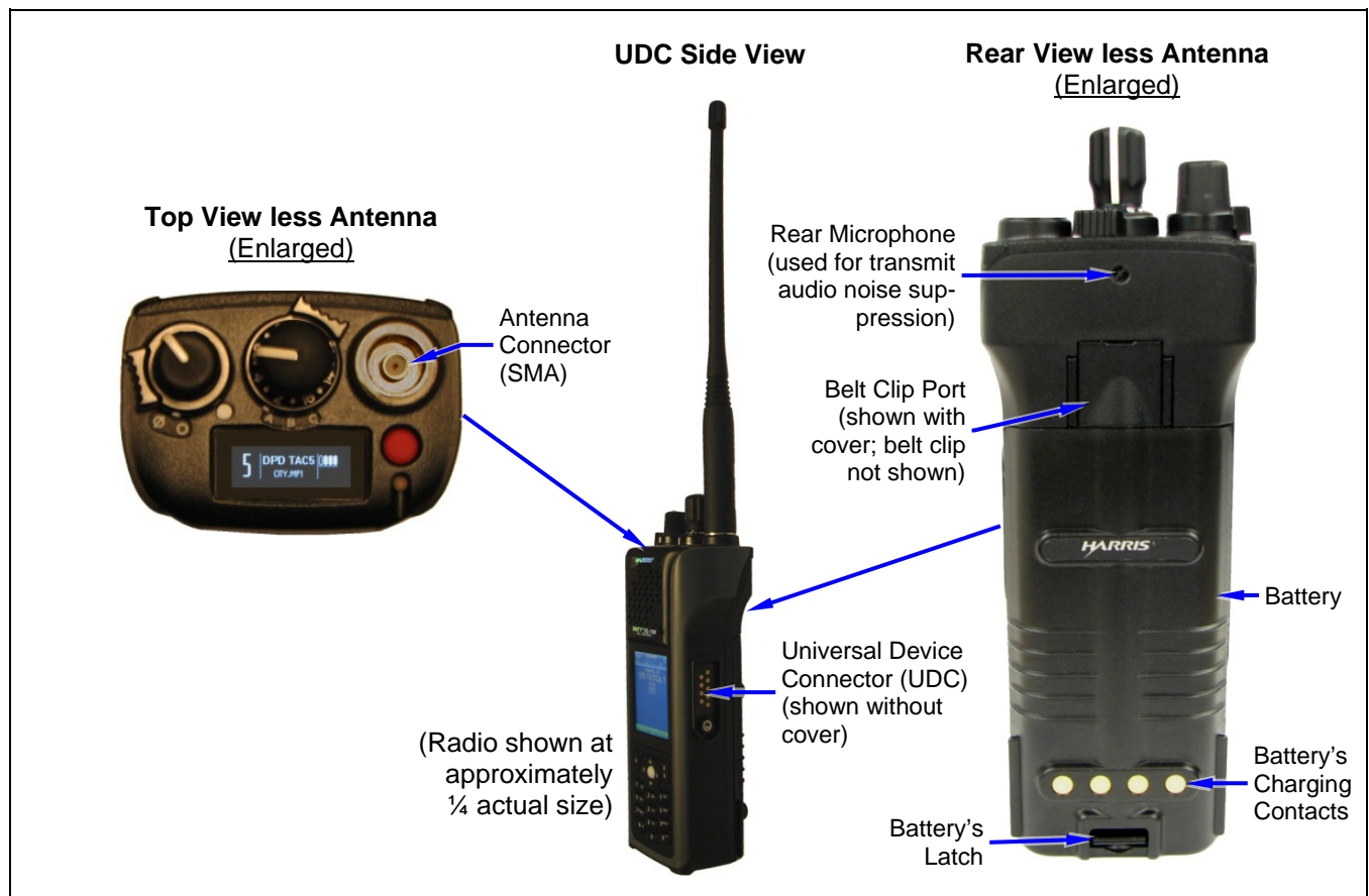
Figure 3-2: Unity XG-100P Portable Radio—UDC Side, Top, and Rear Views
