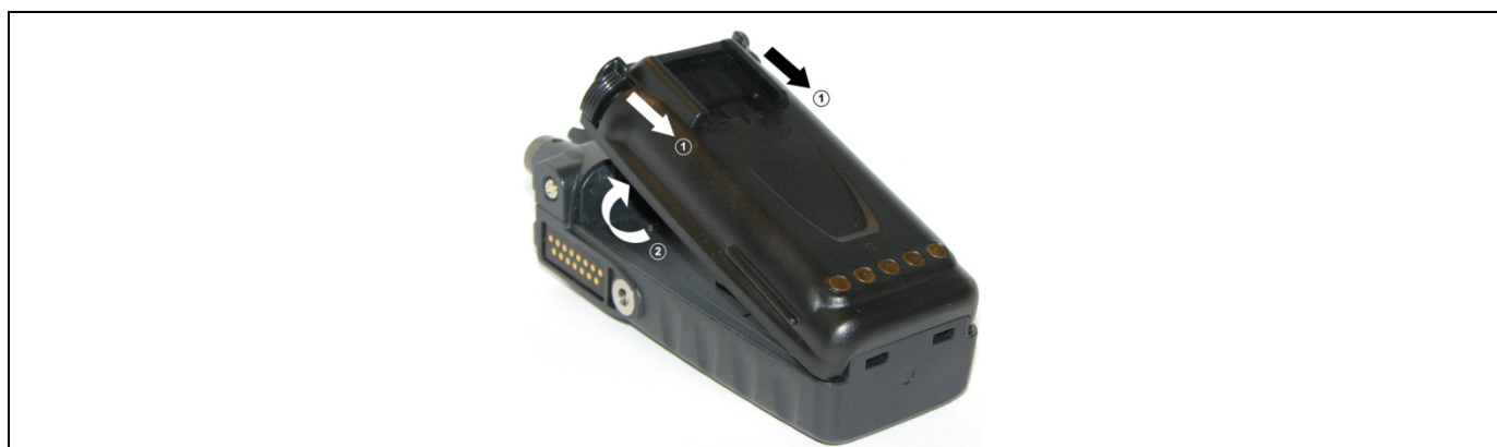
Figure 8-3: Removing the Battery Pack
