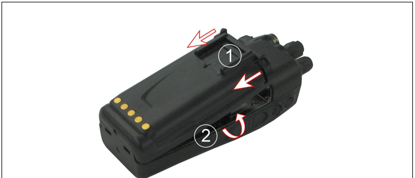
Figure 8-2: Removing the Battery Pack
