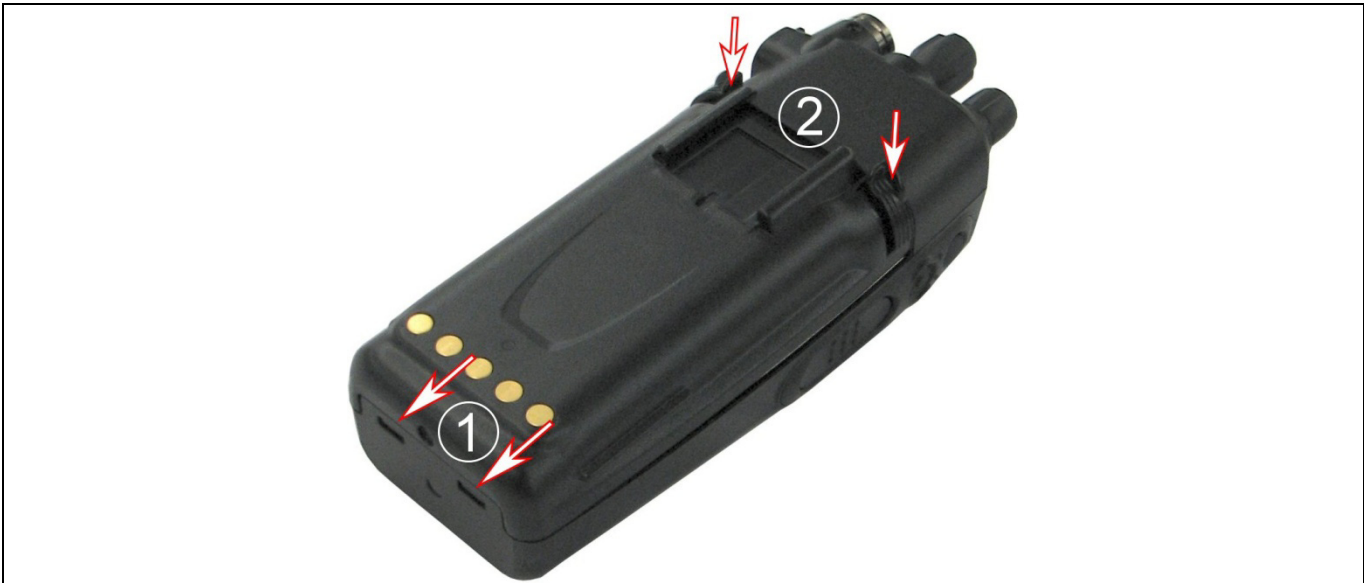
Figure 8-3: Attaching the Battery Pack
