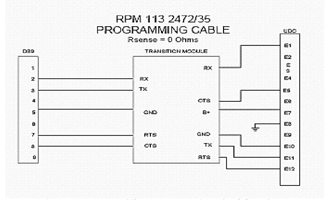
Programming cable has a Zero (Ø) Ohm short on Pin E8 (UDC Sense).
