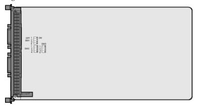
Figure 4-34 DIP switch on the UTRPb4
