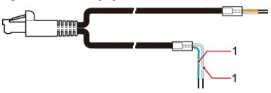
(1) Monitoring signal cable for the PSU (DC/DC)
