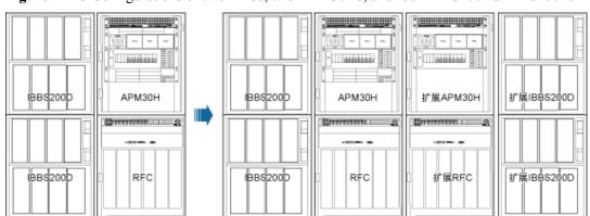
Figure 12-45 Configurations of two RFCs, two APM30Hs, and four IBBS200Ds/IBBS200Ts
