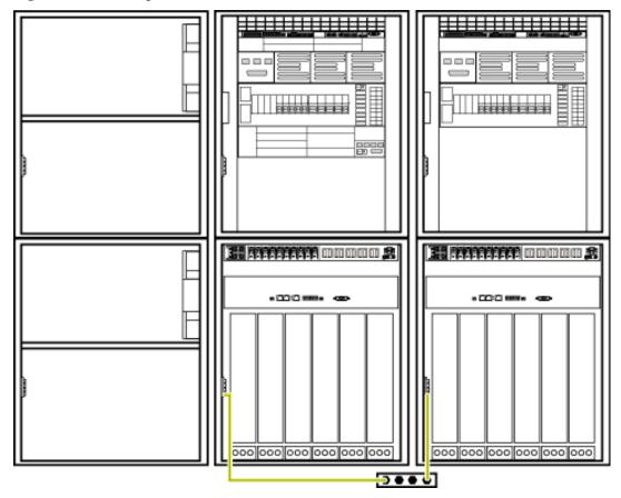
Figure 10-2 Installing the PGND cable
