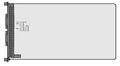
Figure 5-34 DIP switch on the UTRPb4
