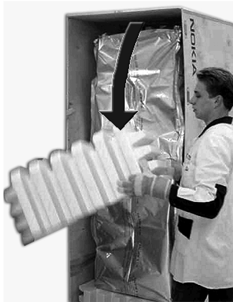
Figure 19. Remove the EPE paddings, first upper, then middle.
