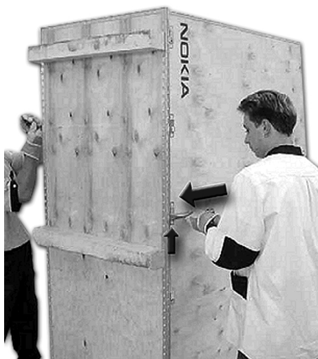
Figure 17. Remove the latches of the bottom plate. To remove the bottom plate bend and remove the latches by using a hammer (or a screw driver).
