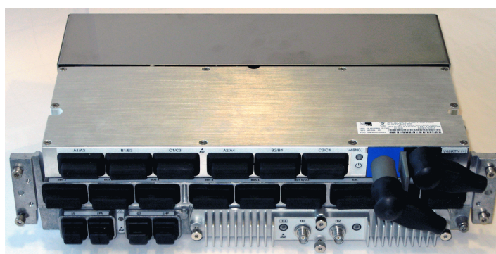
Figure 8. FIFA Flexbus Transmission Sub-module for Nokia Flexi EDGE BTS integrated into Nokia Flexi EDGE System Module (ESMA)
