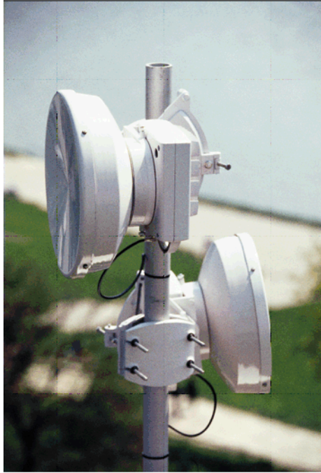
Figure 1. Nokia FlexiHopper (Plus) outdoor unit
