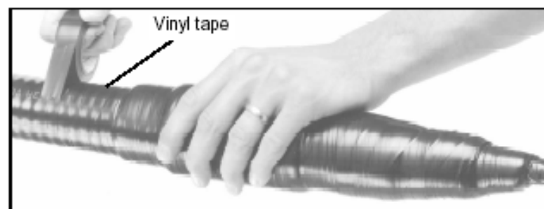
Standard Connector/Splice Weatherproofing Kit
