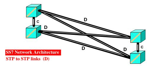
The resulting links are therefore called **Diagonal** or **D** links. In the drawing above the local STP pair is shown on the right at the "lower" level of the hierarchy. The **D** nomenclature makes it unnecessary to add that the STPs connected are not at the same level of hierarchy.
