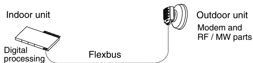
Figure 3. The basic Nokia FlexiHopper network element configuration, one indoor unit and one outdoor unit
