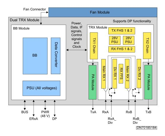
In 2-way diversity case the signal comes from DTRX's other Rx main connector and with 4-way diversity the signal comes from the diversity Rx connector.
