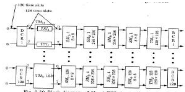
Fig.20.7 Block diagram of No.4 ESS time and space stage.
