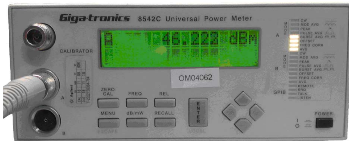
Figure 35 Typical BTS Output power measurement result for By-pass configuration at power level 0 with Giga-tronics 8542C
