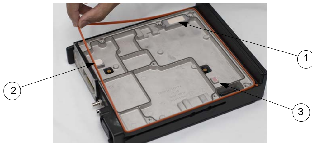
Figure 8-28. All 3 thermal pads located on transmitter (TX) side of main chassis. See Table 8-2 .
