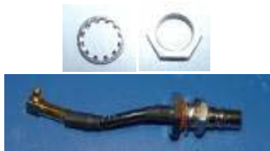
Figure 8-30. Removing the QMA Lock Washer and QMA Nut
