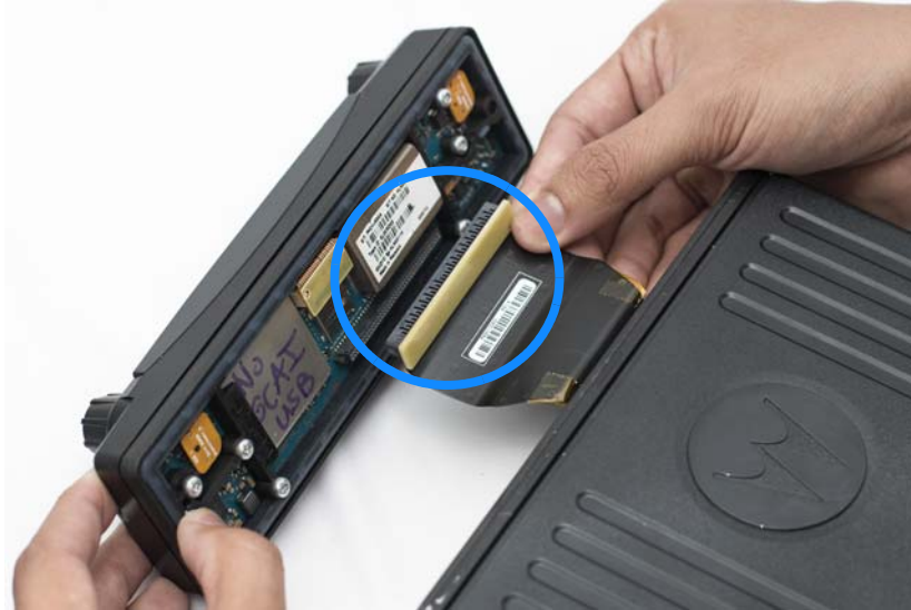
Figure 8-4. Removing the Control Head Flex
