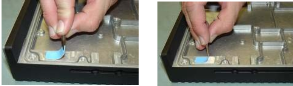
Figure 8-25. Placing Thermal Pad (7575935B01) transmitter (TX) side of main chassis
