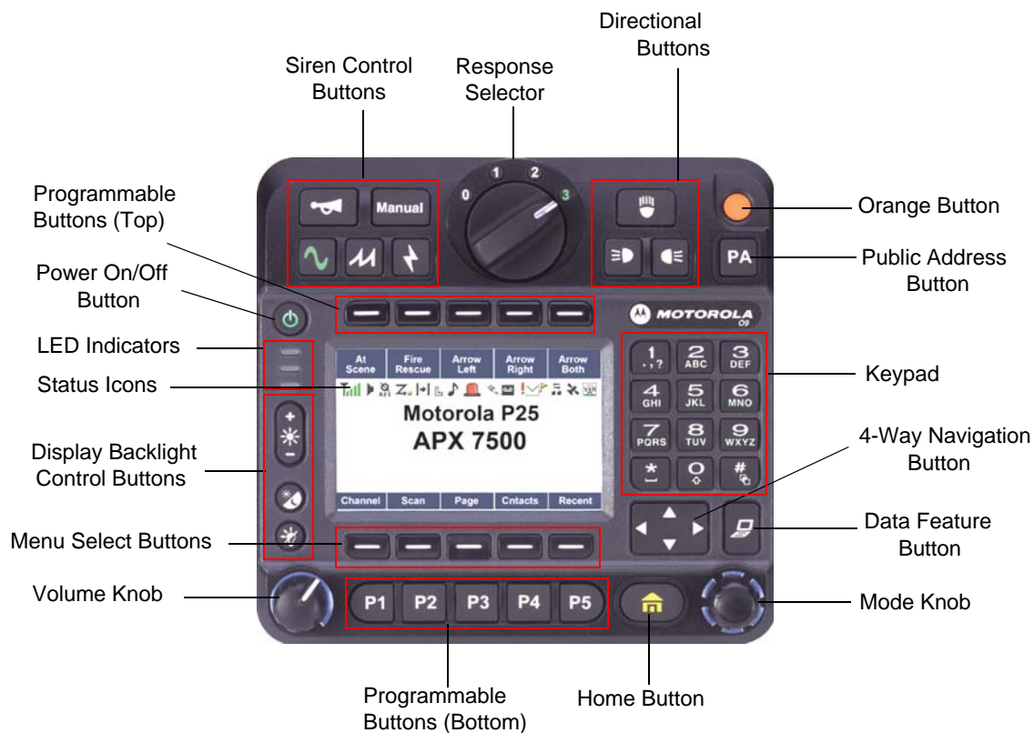
Figure 5-6. O9 Control Head
