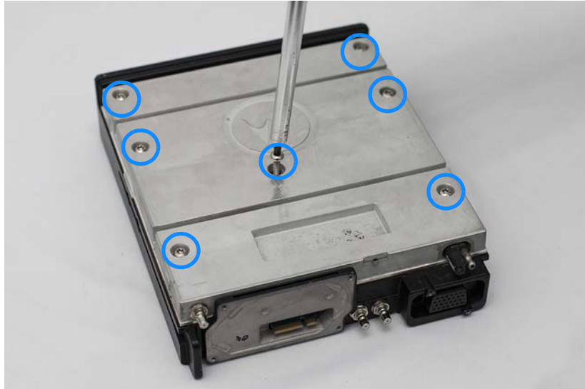
Figure 8-7. Removing the TX Casting Screws
