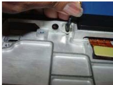
Figure 8-31. Installing two RF Cables into the Main Chassis
