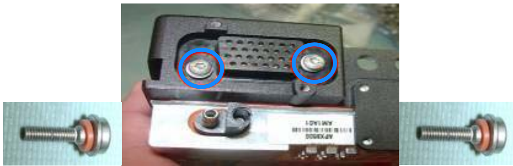
Figure 8-33. Installing Accessory Connector Screws
