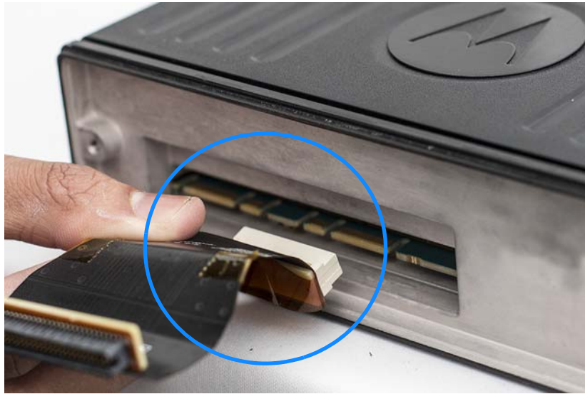
Figure 8-57. Installing Flex into Controller PCB
