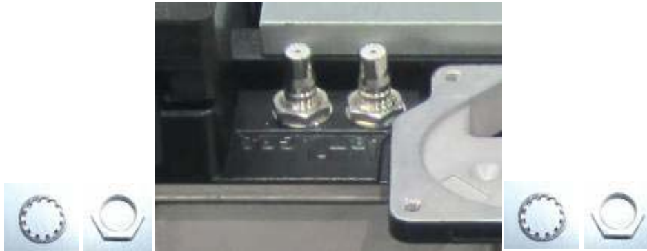
Figure 8-34. Installing the two RF Cables
