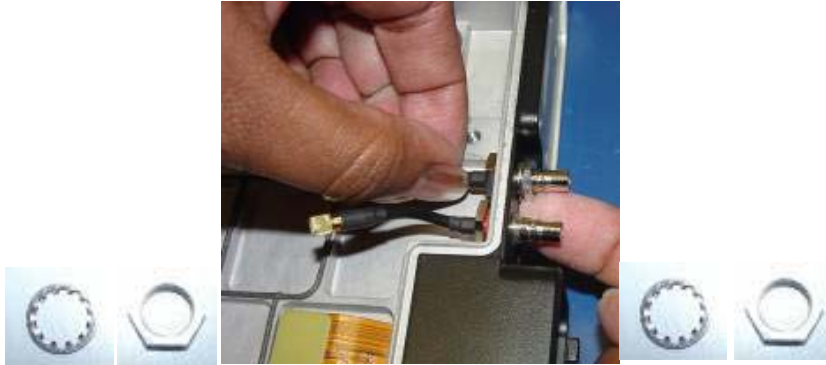
Figure 8-32. Installing QMA Lock Washer and QMA Nut for each cable connector
