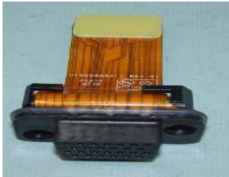
Figure 8-29. Installing the Accessory Connector Flex into Main Chassis
