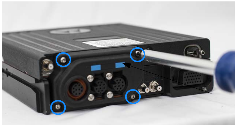
Figure 8-5. Removing the TIB Screws
