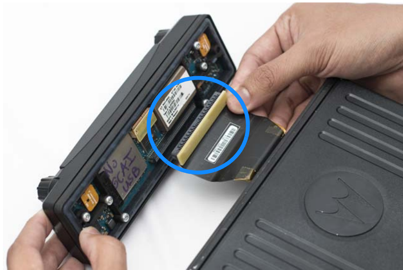
Figure 8-58. Installing Flex into Controller PCB
