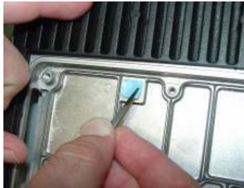
Figure 8-47. Placing Thermal Pad (7575767B01) on transceiver (XVCR) side of main chassis
