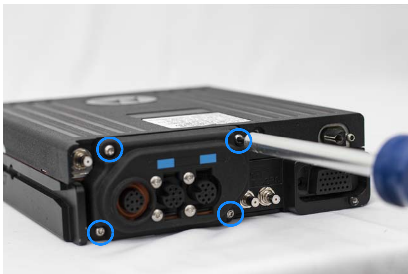
Figure 8-56. Installing the TIB Assembly
