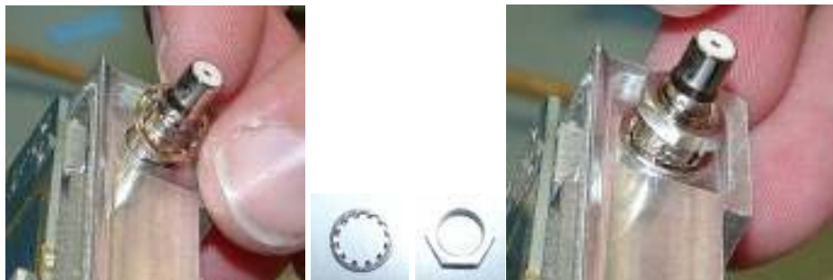
Figure 8-39. Installing the QMA Lock Washer and Nut into the RF Connector
