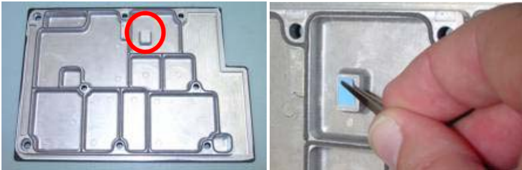
Figure 8-52. Placing Thermal Pad on Transceiver (XCVR) Cover
