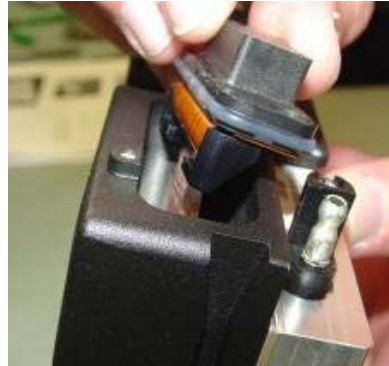
Figure 8-29. Installing the Accessory Connector Flex into Main Chassis
