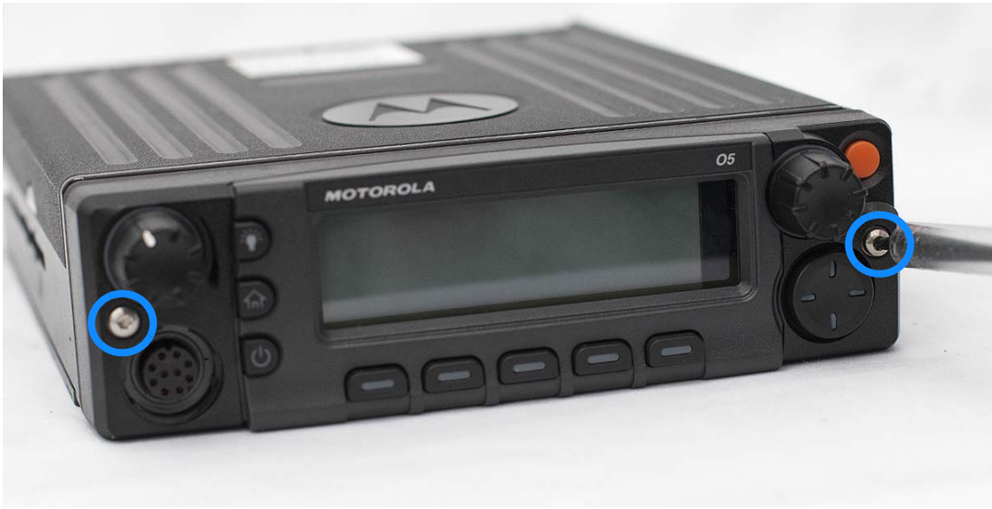
Figure 8-59. Aligning Control Head front of chassis, and Installing the Control Head screws
