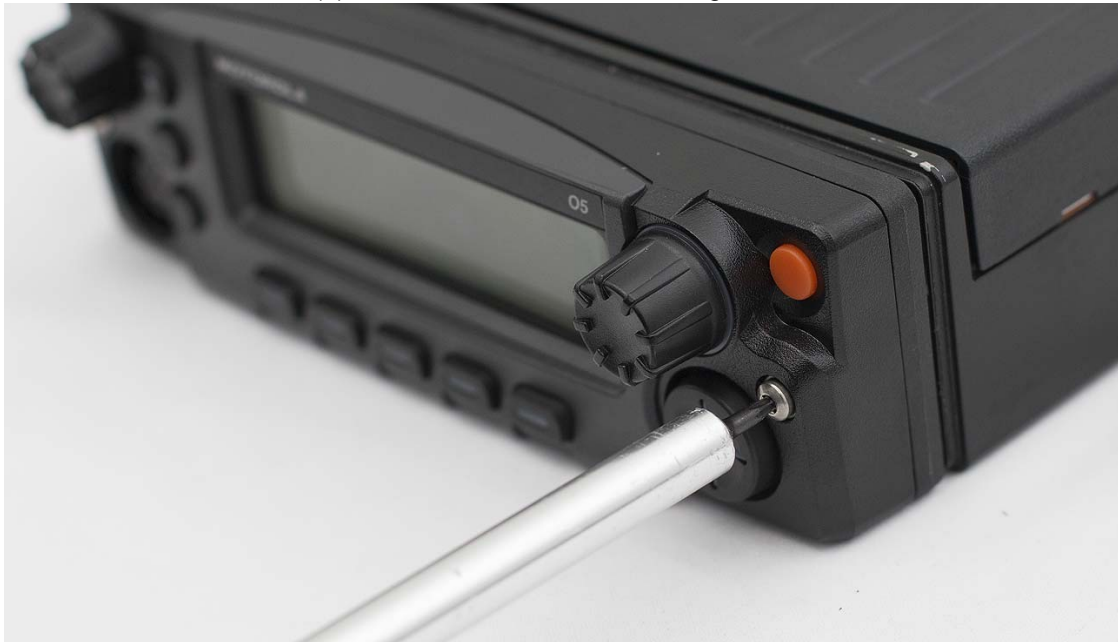
Figure 8-2. Removing the Control Head Screws
