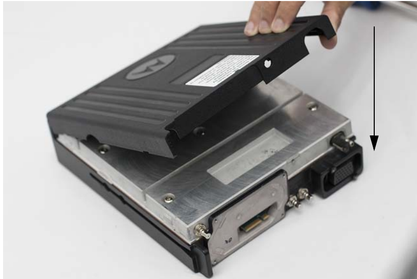
Figure 8-55. Installing the RF Grille
