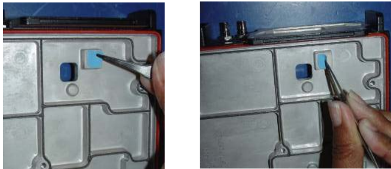
Figure 8-26. Placing Thermal Pad 7575767B01 on transmitter (TX) side of main chassis
