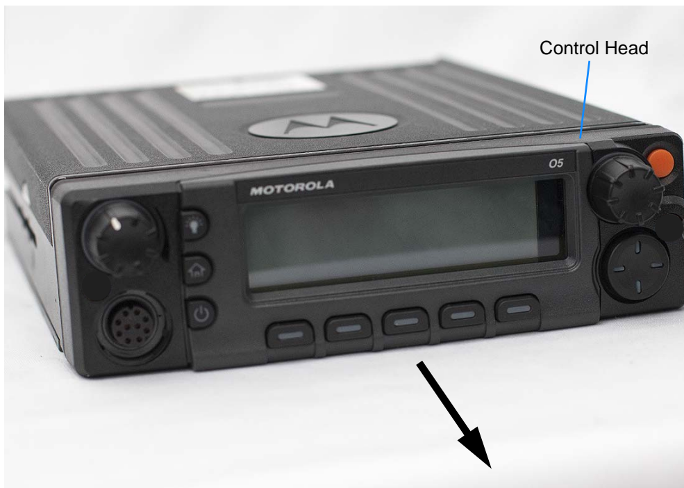
Figure 8-3. Removing the Control Head
