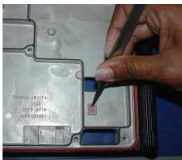
Figure 8-27. Placing the Thermal Pad (HW000572A02) on transmitter (TX) side of main chassis
