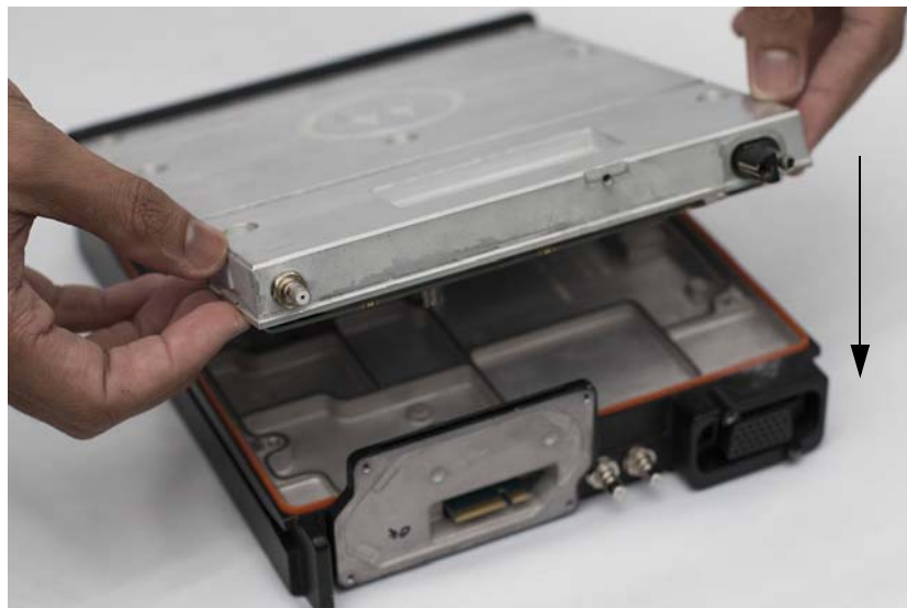
Figure 8-45. Placing Transmitter Cover onto the Main Chassis
