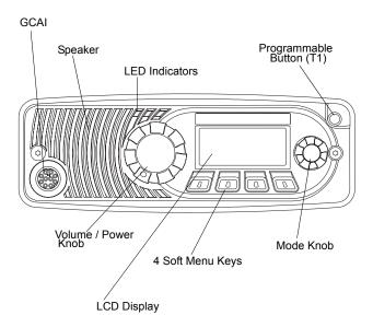
ASTRO XTL 1500 Digital Mobile Radio with Control Head
