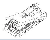
3 Slide battery latch into lock position.
