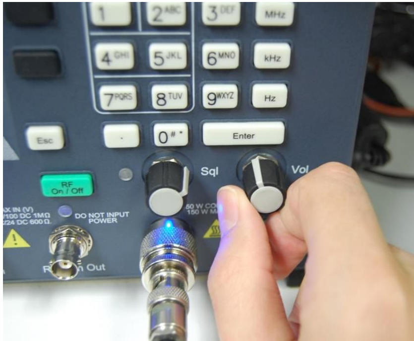
Figure 7-2. Adjust analyzer volume until about 4 kHz deviation is measured.
