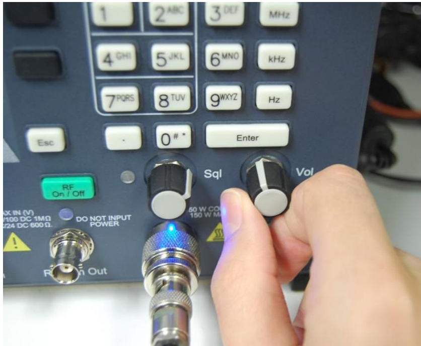
Figure 5-2. Adjust analyzer volume until about 4 kHz deviation is measured.
