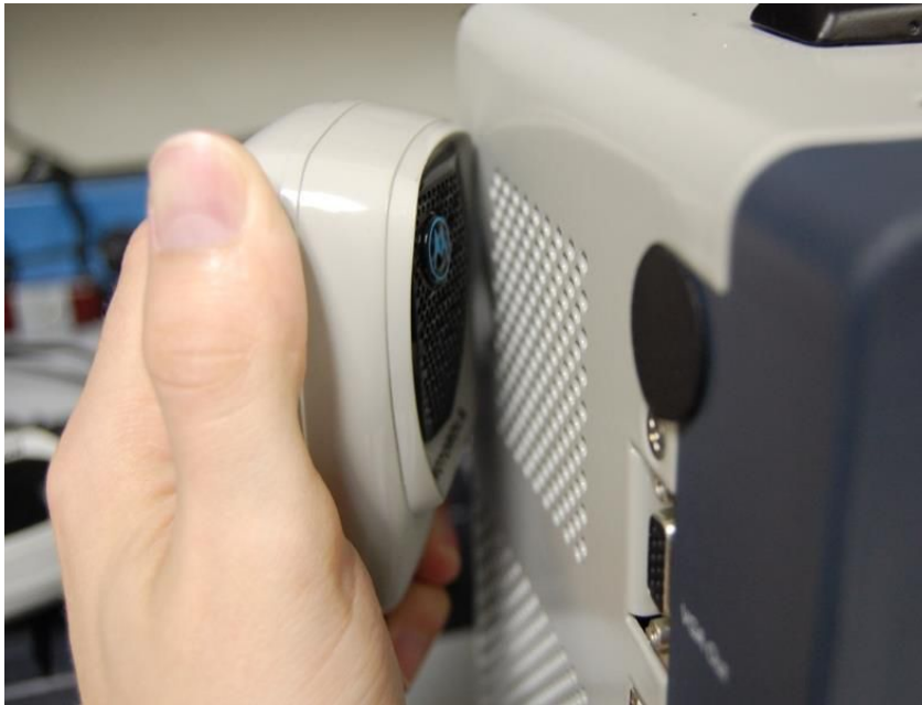
Figure 7-1. Place keyed radio next to analyzer speaker.
