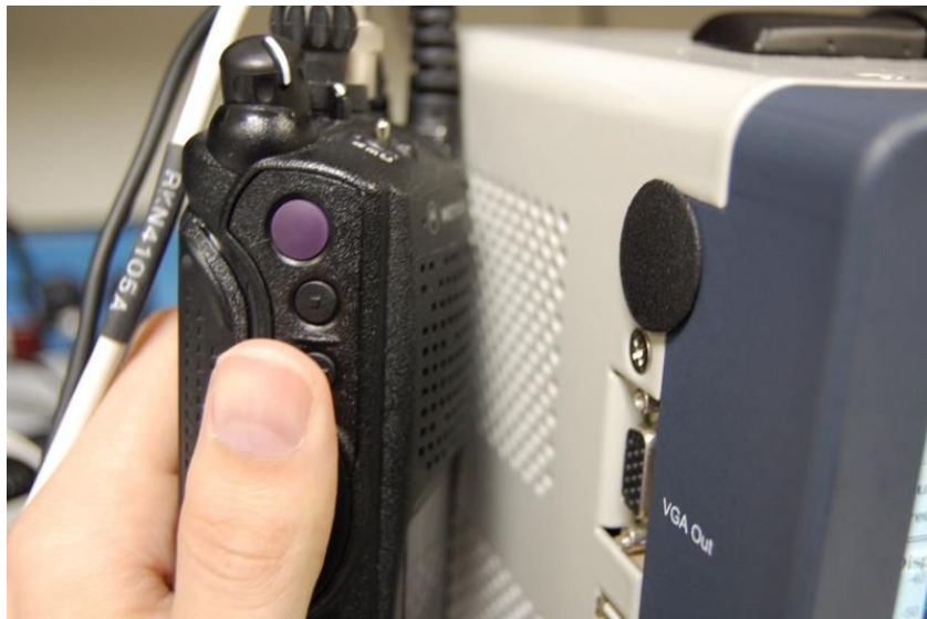
Figure 5-1. Place keyed radio next to analyzer speaker.
