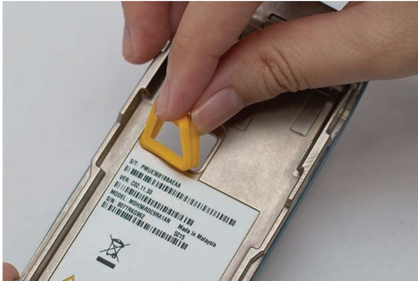
Figure 5-12. Battery contact seal removal
