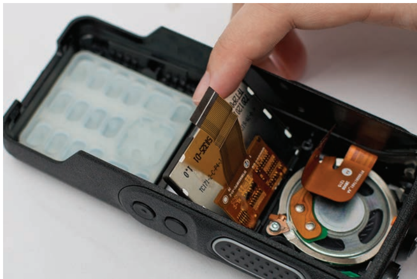
Figure 5-19. Display module removal
