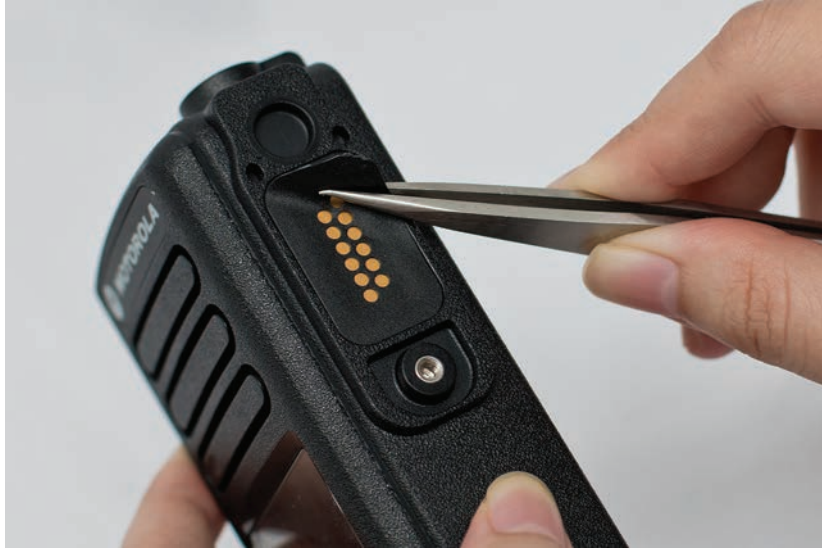
Figure 5-30. UC Escutcheon replacement
