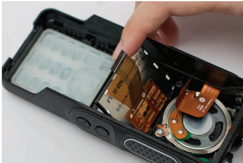
Figure 5-31. Display module reassembly
