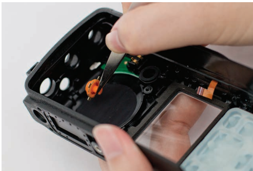
Figure 5-27. Emergency button reassembly
