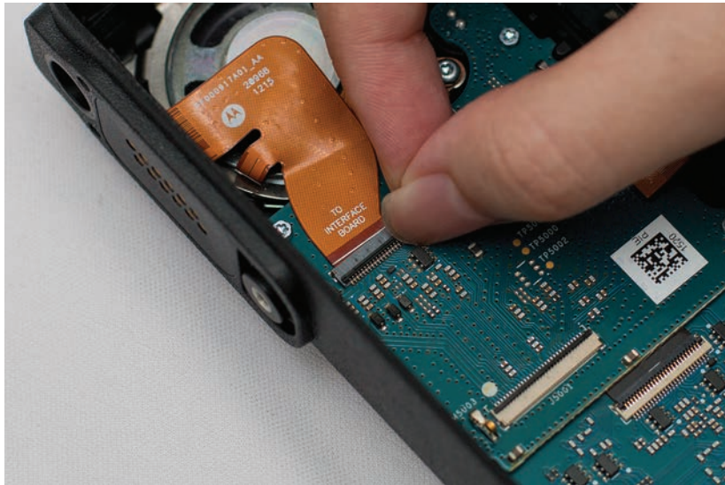
Figure 5-15. UC flex removal
