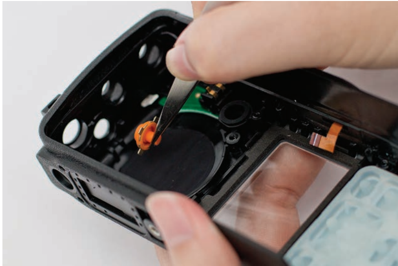
Figure 5-24. Emergency button removal
