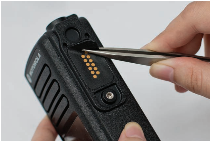
Figure 5-20. UC escutcheon removal
