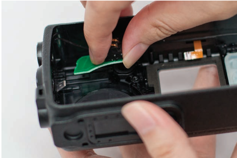
Figure 5-26. Bluetooth GPS antenna reassembly
