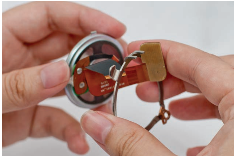
Figure 5-28. Speaker retainer reassembly
