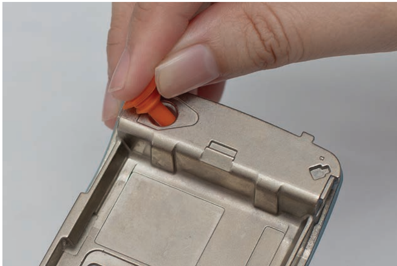
Figure 5-13. RF rubber plug removal
