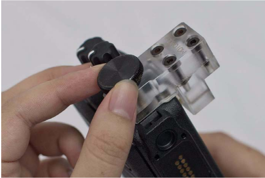
Figure 4-5. RF Adaptor screw
