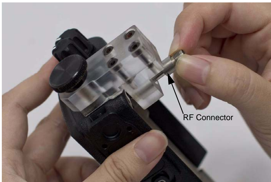
Figure 4-6. RF Adaptor complete assembly
