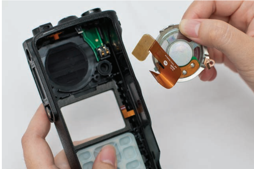
Figure 5-22. Speaker assembly removal
