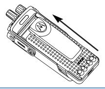
**2** To remove the battery, turn the radio off. Move the battery latch marked **A** into unlock position and hold, and slide the battery down and off the rails.
