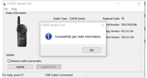
7. Ensure the radio model is the one you want to upgrade and with correct firmware version which is R01.01.00 in this example. Do not proceed update if the radio is not the correct model/firmware version.
