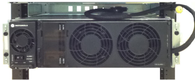
Figure 130: Analog Simulcast Cable – GTR 8000 Base Radio with Fan Modules
