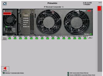
When an alarm condition occurs, the alarm box for one of the modules begins to flash red. Selecting the LED box opens an alarm pop-up window indicating details of the alarm. To view the status of all alarms for a particular module within the device, select the alarm LED box corresponding to the particular module. Alarms can be acknowledged by pressing the **Acknowledge** button on the screen.
