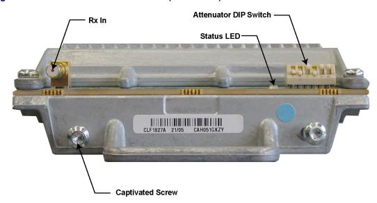
Figure 2-16 Cabinet RMC/LNA Module (Front View)
