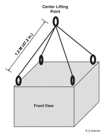
Figure 3-2 Lengths and Angles for Lifting Using the Eyenuts
