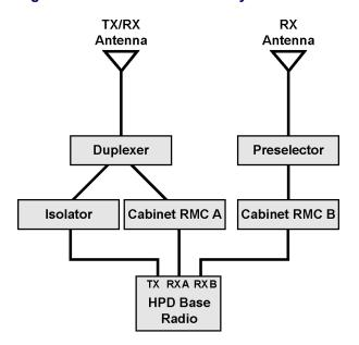
Figure 1-4 GTR 8000 Site Subsystem - Transmit/Receive Paths
