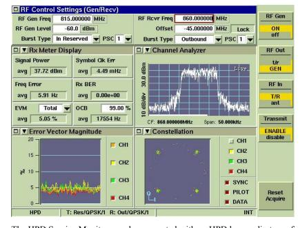
Figure 5-1 HPD Service Monitor - Test Screen (Aeroflex 3900 Series Service Monitor)
