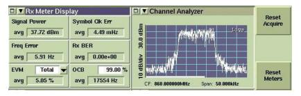
11 Compare the value that displays in the **Signal Power** field to the base radio Tx Power Out specification **that** matches your base radio configuration. See 1.6.1 Specifications for GTR 8000 Base Radio (700/800 MHz), page 1-6 in the Description chapter of this documentation.
