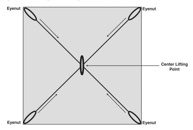
Figure 3-3 Proper Alignment of the Eyenuts
