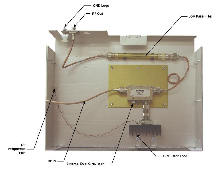
Figure 9-14 Dual Circulator/Isolator Tray (Top View)
