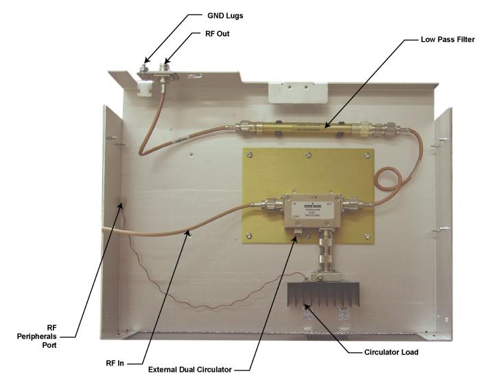
Figure 2-18 External Dual Circulator/Isolator Tray
