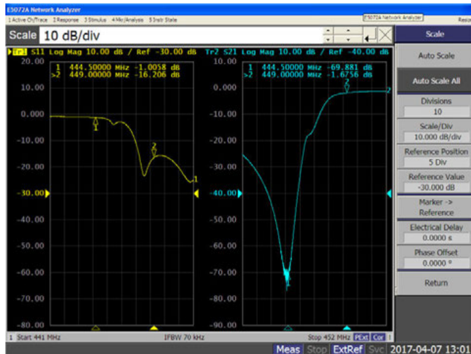
Figure 24: Tuning the HIGH Port of the Duplexer
