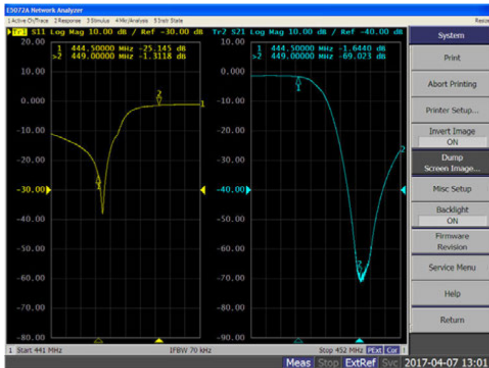
Figure 25: Tuning the LOW Port of the Duplexer
