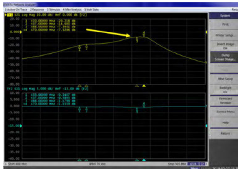
Figure 123: Passband Tuning of Tuning Screw 2 to the New Passband
