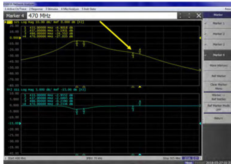
Figure 122: Passband Tuning of Tuning Screw 1 to the New Passband
