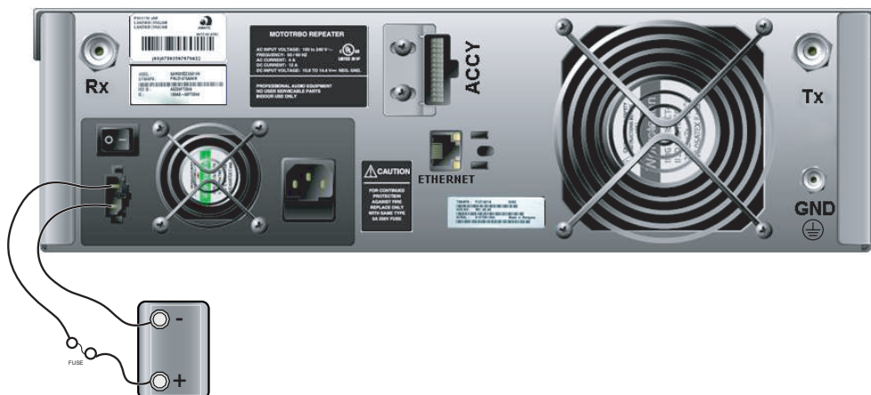
Figure 4-2 Making Connections to a Backup Battery
