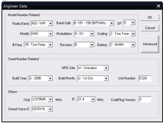
This is where you can change your Minitor V's core settings (i.e. Radio Band (LOW, VHF, UHF), Band Split, Number of Frequencies).
