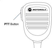
The microphone is activated when the PTT button is pressed.
