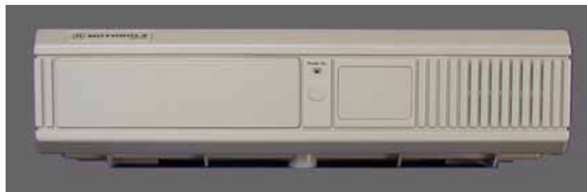
Figure 3-3. Consolette Front Panel—G81 Option
