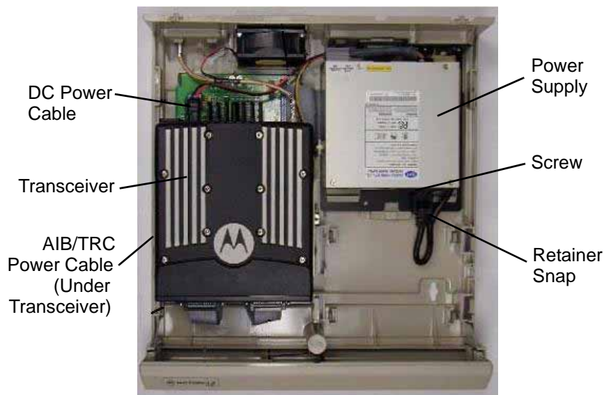
Figure 4-4. Removing the Power Supply
