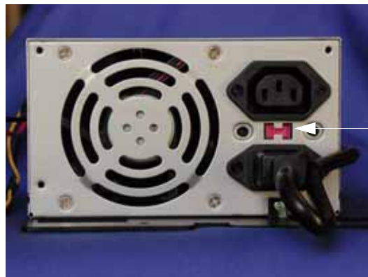
Figure 2-3. Power Supply VAC – Select Switch
