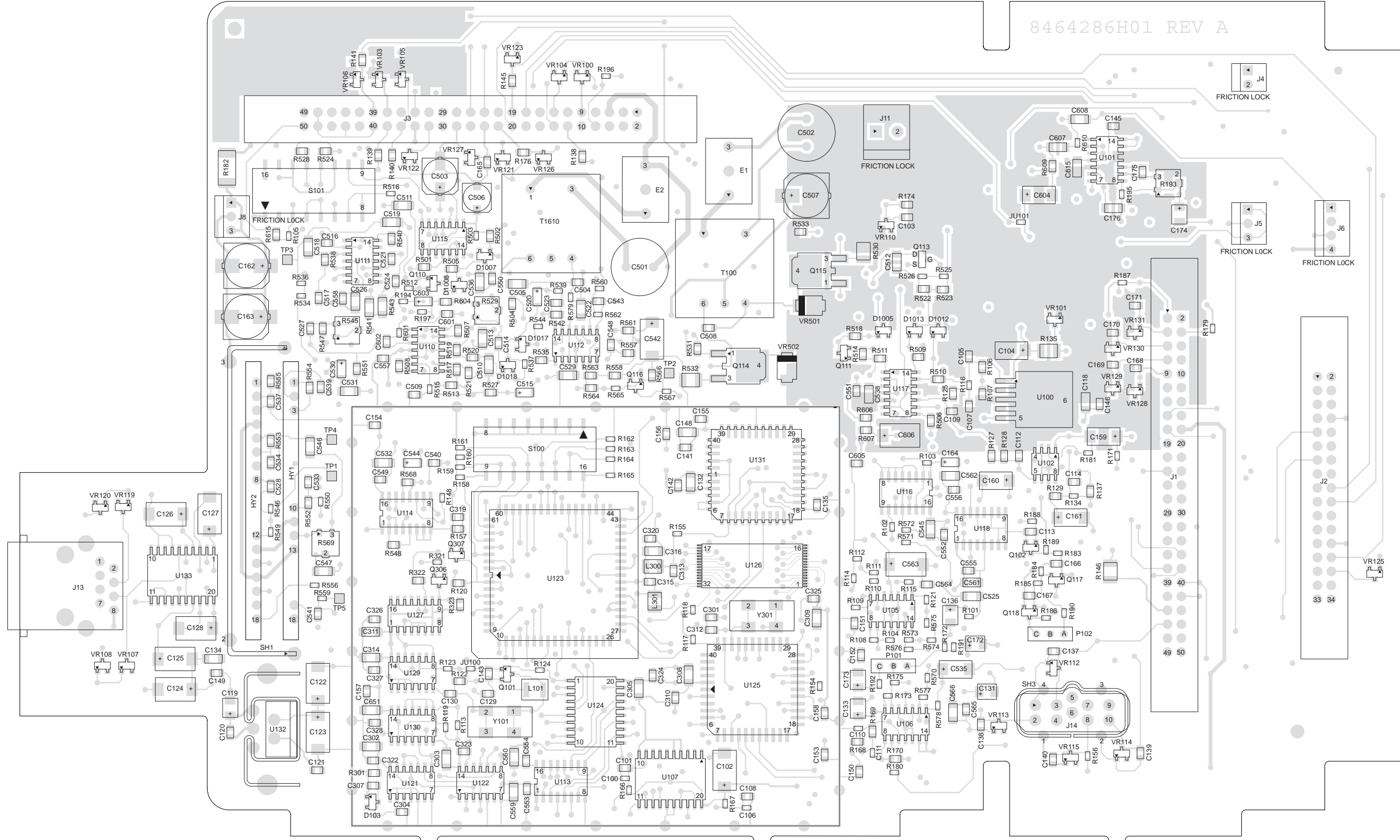
Figure 7-10. PLN1687A Tone Remote Control Board Component Location Diagram (Viewed from Side 1)
