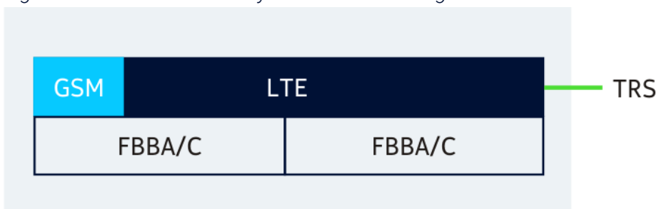
Figure 4: GSM-LTE shared system module configuration
