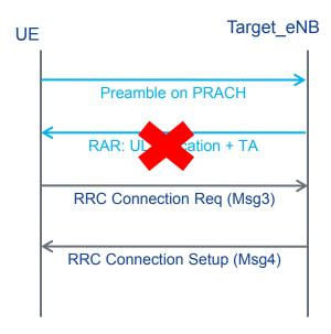
RAR power level itself cannot be changed, but as it is scheduled on PDCCH, its aggregation level can be adjusted by parameter *pdcchAggRaresp* (4,8), default 4.
