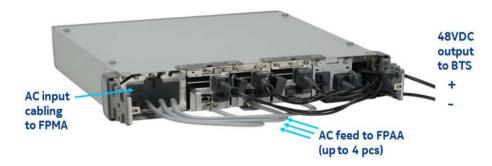
Figure 92: Flexi Power Module FPMA
