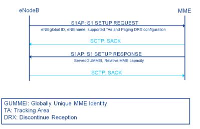
Figure 264: S1 Setup Procedure
