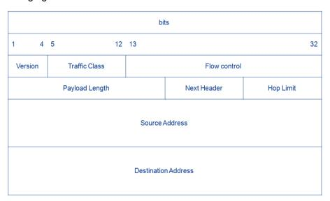
Figure 36: IPv6 Header
