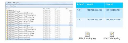
Figure 32: Modules / RRH IP addresses from RL60 onwards
