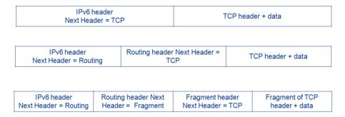
Figure 37: IPv6 Header extensions
