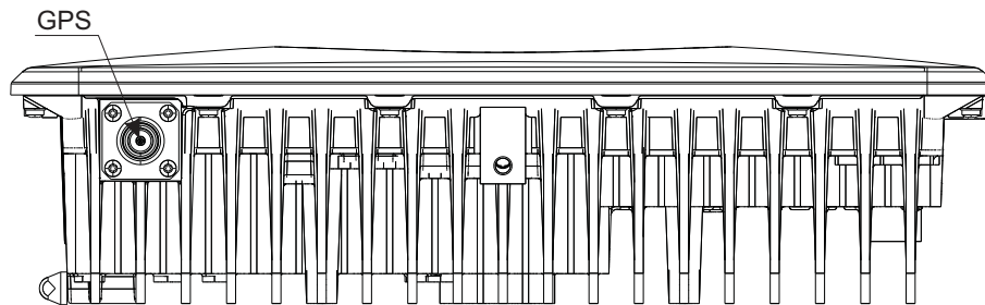
Figure 9 Flexi Zone Micro BTS (FWGB, FWHA, FWIB) side view interfaces
