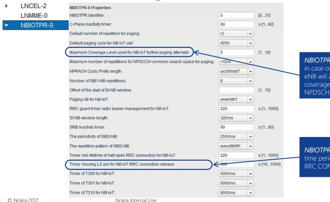
NBIOTPR:pagAttMaxCovNB indicates a threshold in case of Paging Attempt Count greater than this, eNB will apply the highest (maximum) configured coverage level parameters for NPDCCH and
