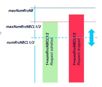
Please note: numRrcNBCL1/2 are the RAC counte for consumed RRC connections for NB-IoT UEs in coverage level 1 and 2 \*numRrcNB is an RAC internal counter to keep track of admitted NB-IoT UEs
