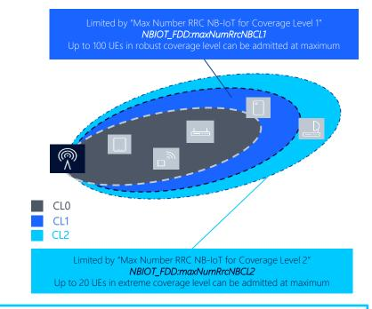
Moreover in addition to RAC checks against *maxNumRrcNBCL1* and *maxNumRrcNBCL2* thresholds, check against *NBIOT\_FDD:maxNumRrcNB* threshold which limits max number of RRC Connected NB-IoT users per NB-IoT cell must be done as well.
