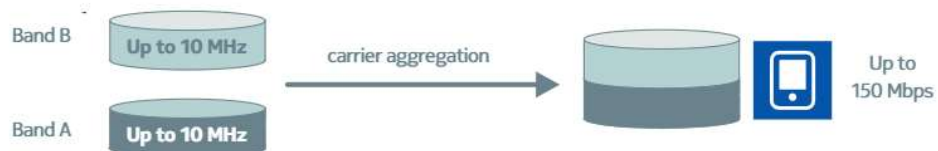
Figure 12 Inter-band carrier aggregation example
