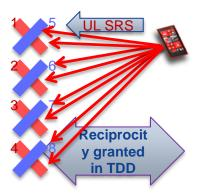
In TDD, radio pilot overhead depends on the number of spatially multiplexed UEs. It does not depend on the number of the antennas.
