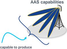
mMIMO AAS is capable to produce more than just one beam each beam can potentially serve one UE
