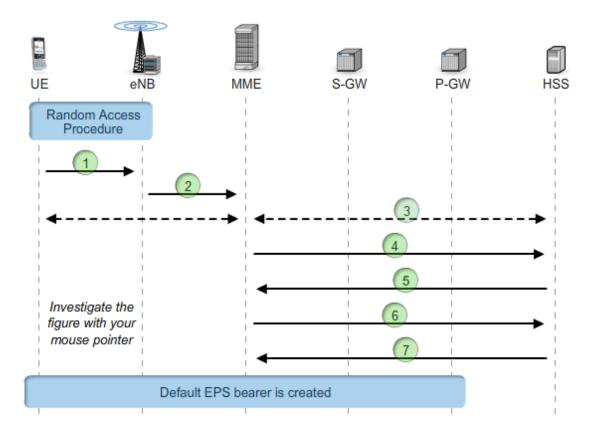
The random access procedure is necessary for establishing an RRC signalling connection between UE and eNB.
