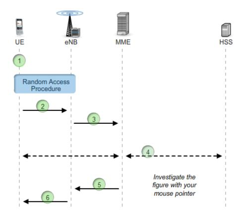
1. The UE detects a change to a new tracking area (TA) by discovering that the current TA indicated on the broadcast channel is not in the list of TAs that the UE registered with the network.
