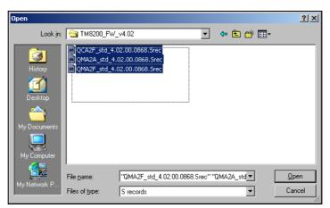
Click Open and the process will continue. Each file will write to the radio body and control head in sequence
