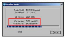
After serial number 19257949 in April 2007 TM8100's are built with 2C5 FPGA's and these are identified with Hardware v02xx.
