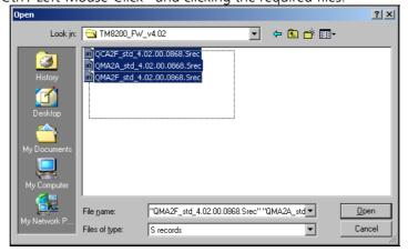
Click Open and the process will continue. The files will write to the radio body and control head in sequence.
