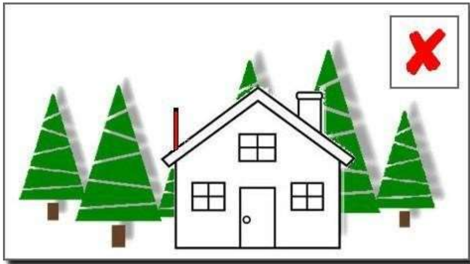
Figure 2 - Bad Position. Roofline and Trees Block Data
