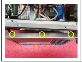
Remove 3 screws from the top edge of the flap.
