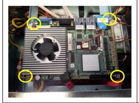
Remove the screws (2 in total) and spacers (2 in total) that bind the SBC to the frame.
