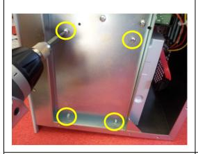
Remove the screws (4 in total) that bind the disc drive to the enclosure frame.
