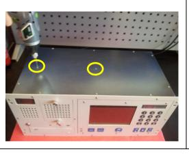
Fit the two screws that hold the stack of analogue channel cards first.
