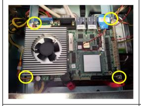
Replace the screws (2 in total) and spacers (2 in total) that bind the SBC to the frame.
