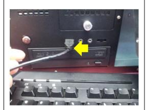
Connect a USB keyboard to the external USB port.
