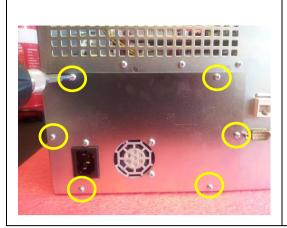
Replace the screws (6 in total) that bind the power supply cover plate to the enclosure frame.
