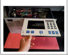
To remove the keyboard and LCD face plate you must lift the screen flat to its highest up-right position.
