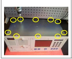
Remove the rest of the screws (10 in total) that hold the top cover plate in place.
