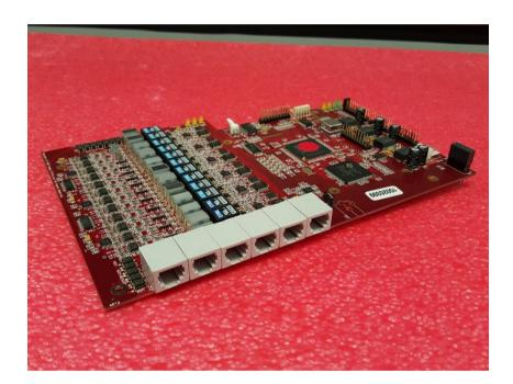
Its function is to interface analogue audio lines and analogue telephone lines to the Total Recall VR for the purpose of recording.
