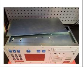
Finally, simply remove the bottom cover plate.
