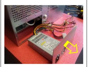
Remove the power supply (with the cover plate) from the enclosure.
