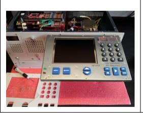
To fit the keyboard and LCD face plate you must lift the screen flat to its highest up-right position
