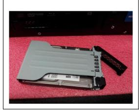
Replace the faulty drive with the new one.
