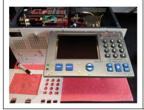
The unit without its keyboard and LCD face plate.
