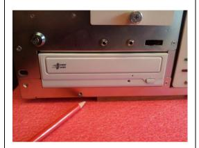
Sit the unit on top of the spacer and make sure that the front bottom edge is above the bench surface.
