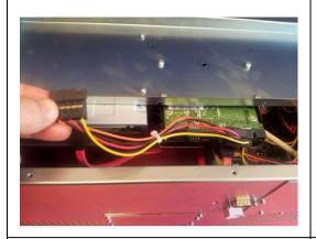
Disconnect the power cables from the disc drive and the hard disk.
