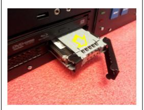
Use the front arm of the bracket to disconnect the dive and pull the bracket out.
