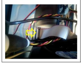
Attach the keyboard cable to the midboard.
