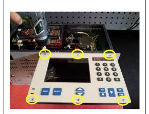
Remove the screws (6 in total) that hold the face plate in place.
