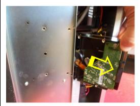
Simply remove the hard disk from the enclosure.
