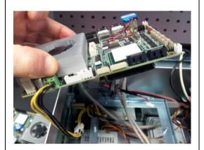
Carefully place the new SBC in position. Be careful to leave all cables above the SBC.
