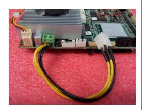
Attach the power cable to the new SBC.
