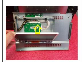
Lift the LCD panel and place it its frame.
