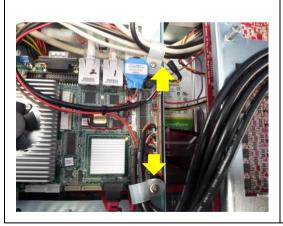
Remove the P clips (2 in total) that attach cables to the edges of the SBC.
