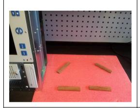
To fit the main face plate you must sit the unit at a small distance from the bench surface.
