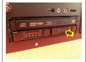
Use the arm to connect the disk to the system and lock in place.
