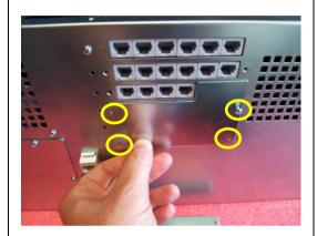
Install the port blanking plates(s) – if removed.
