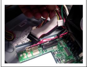
You will be able to reconnect the keyboard ribbon cable, mid-board power cable and LCD inverter power cable now.
