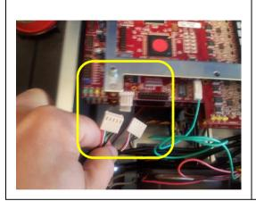
Disconnect the USB cables from all analogue channel cards.
