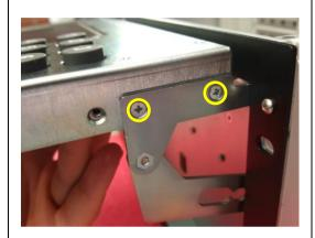
Detach the flap from the right pivot arm by removing the screws (2 in total) that bind the flap to the arm.
