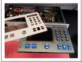
Remove the face plate while making sure that the flap remains in its up-right position.
