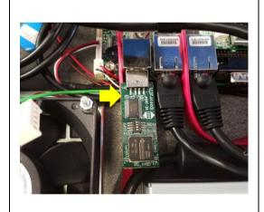
Remove the old AMBE decoder and attach the new AMBE decoder to the top external USB port on the SBC.
