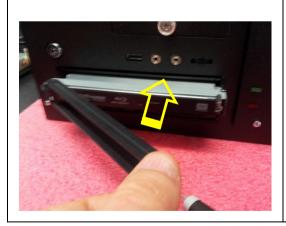
Use the arm of the bracket to connect the disc drive to the system and lock it in place.
