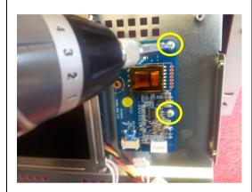
Remove the screws (2 in total) that bind the inverter to the enclosure.
