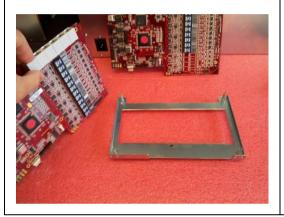
Remove the card that will be replaced. Put this card aside so you do not mix it up with the new card.
