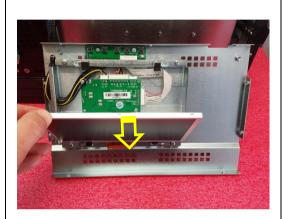
Separate the LCD panel from the frame by lowering the top edge and keeping the bottom edge on the fame.
