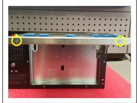
Remove 2 screws from the bottom edge of the flap.
