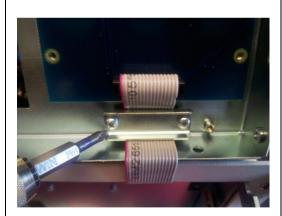
Replace the cable clamp that holds the keyboard cable.
