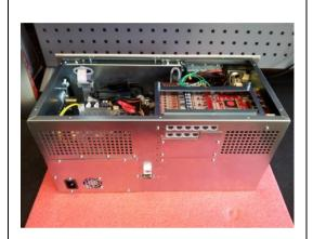
It is easier to remove the stack of analogue channel cards if you are facing the back of the unit.
