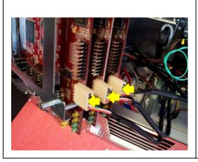
Attach a USB cable to J23 on each of the cards.
