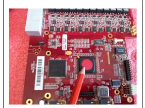
Make sure that the new card has the same colour sticker on the FPGA chip as the other cards in the stack.
