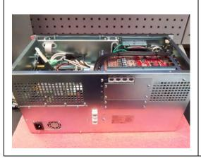
It is easier to replace the SBC if the back of the enclosure is facing you.
