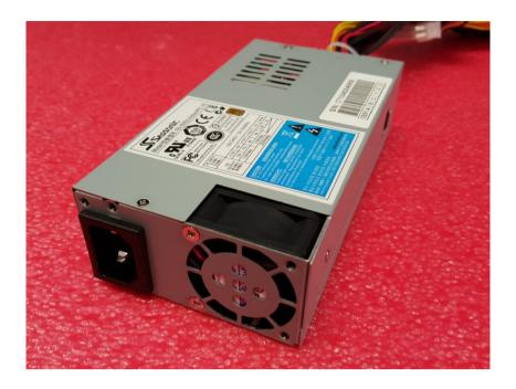
The position of the fan is not the same on all Flex form factor power supplies. If you source your own power supply you may find that the fan hole on the enclosure partially covers the fan.
