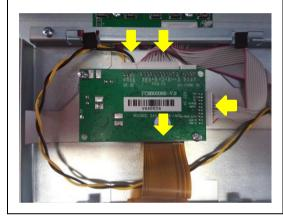
Connect the all cables to the VGA driver board.
