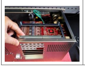
Place the stack in its position in the enclosure.
