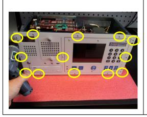
Place the face plate in position and then replace the screws (13 in total) that bind the face plate to the main enclosure.
