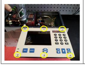
Replace the screws (6 in total) that hold the face plate in place.
