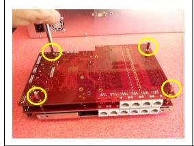
Attach it to the stack with the spacers.
