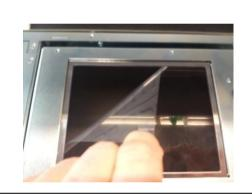
If you installed a new LCD screen then peel the screen protector from the face of the screen.
