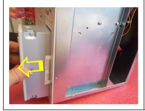
Simply remove the disc drive from the enclosure.
