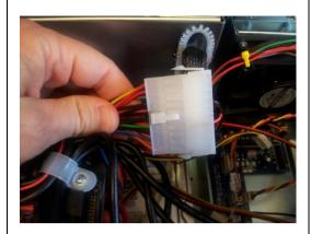
Locate the on/off key switch connector. It may be hidden under the SBC and close to the power supply.
