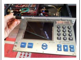
Remove the glass cover plate which protects the LCD screen.
