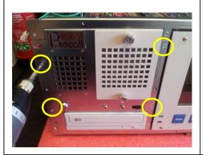
Put the whole sub-assembly back into the enclosure.
