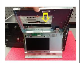
Join the keyboard from the monitor assembly by lowering the keyboard assembly from its lower edge.
