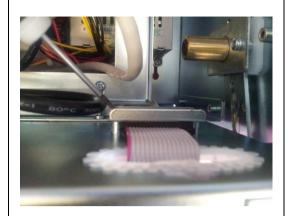
Replace the cable clamp that holds the keyboard cable on the inside wall of the enclosure.
