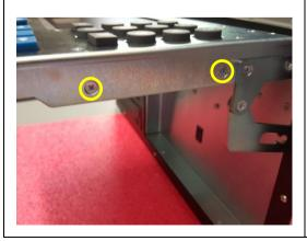
Remove 2 screws from the left edge of the flap.
