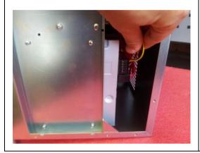
Attach the SATA and power cables to the disc drive.
