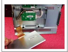
Now you can separate the LCD panel from the rest of the assembly.
