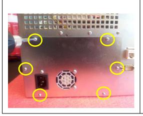
Remove the screws (6 in total) that bind the power supply cover plate to the enclosure frame.
