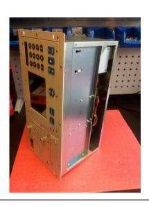
It is easier to replace the disc drive if you sit the unit on its side.
