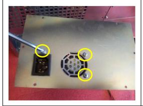
Remove the screws (3 in total) that bind the cover plate to the power supply.
