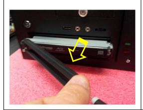
Use the arm to disconnect the disc drive from the system and pull it out.
