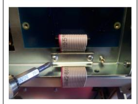
Remove the cable clamp that holds the keyboard cable.
