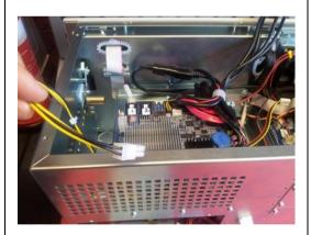
Route the power feed for the SBC to the left side of the enclosure.
