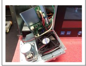
You should be able to pull the whole assembly out with the remaining cables attached to the mid-board.
