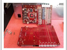
Carefully separate the last card from the stack.
