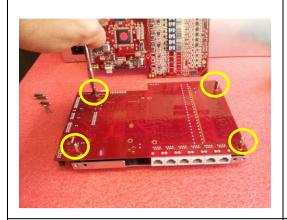
Remove the spacers which hold the card that will be replaced.
