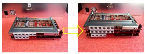
Note that, as an example, during the procedure we will move the card with 8 channels from position 2 in the stack to position 3. The new 12 channel card will take position 2. Typically you will simply add the new card as the last card in the stack.
