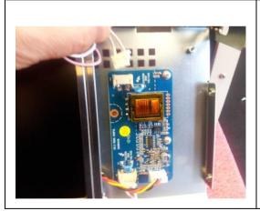
Disconnect the LCD screen from the inverter.
