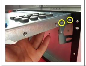
Lift the flap fully upright and bring its top right corner near the right pivot arm.
