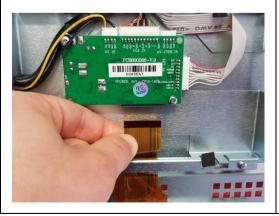
Disconnect the TTL cable from the VGA driver board.
