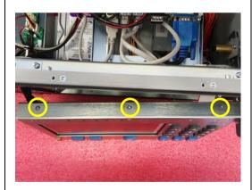
Replace 3 screws on the top edge of the flap.
