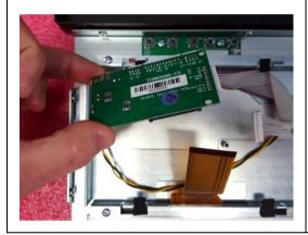
Separate the driver board from the frame.
