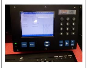
Turn the system on and while it is starting press the Delete key on the keyboard to enter the BIOS setup program.
