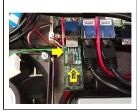
Attach the AMBE decoder to the top external USB port on the SBC.
