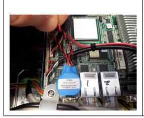
Simply disconnect the old battery and connect the new one.
