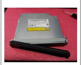
Replace the faulty drive with a new one.
