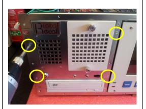
Remove the screws (4 in total) that bind the sub-assembly to the main enclosure.
