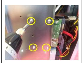
Replace the screws (4 in total) that bind the hard disk to the enclosure frame.
