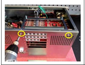
Replace the screws (2 in total) that attach the frame to the enclosure wall.
