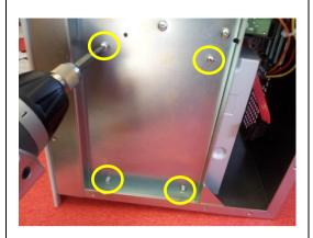
Replace the screws (4 in total) that bind the disc drive to the enclosure frame.
