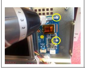
Place a new inverter in position and replace the screws (2 in total) that bind the inverter to the enclosure.
