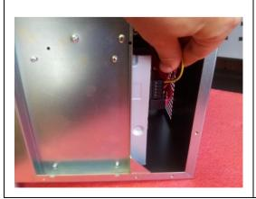
Disconnect the SATA and power cable from the disc drive.
