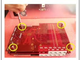
Remove the spacers which hold the last card in the stack.
