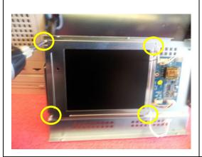
Remove the screws (4 in total) that bind the screen to the enclosure.
