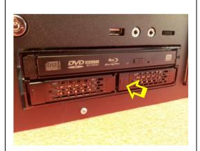
Push the latch on the side of the hard disk bracket to release the bracket.
