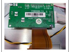
Attach the TTL cable to the VGA driver board.
