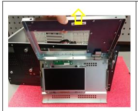
Separate the keyboard from the monitor assembly by lifting the keyboard assembly from its lower edge.
