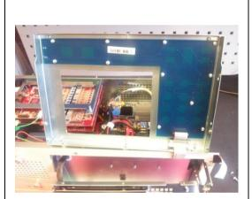
Sit the top part of the sub-assembly (the part with the keyboard) on the top edge of the system.
