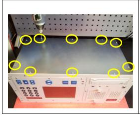
Remove the screws (10 in total) that hold the bottom cover plate in place.
