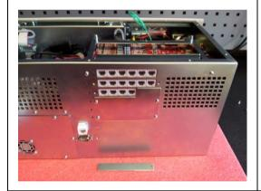
The unit with the stack of analogue channel cards in place.
