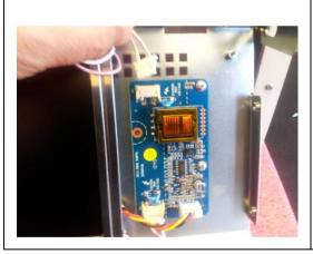
Disconnect the LCD screen from the inverter.
