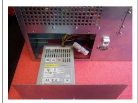
Insert all cables into the enclosure, but do not insert the power supply.
