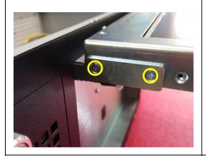
Detach the flap from the left pivot arm by removing the screws (2 in total) that bind the flap to the arm.
