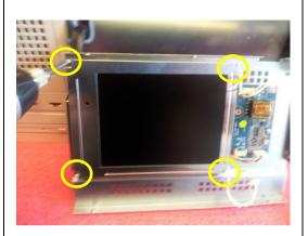
Place the screen in position and replace the screws (4 in total) that bind the screen to the enclosure.
