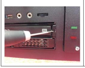
Use a small screwdriver to release the latch that holds the arm of the bracket that houses the disc drive.
