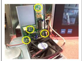
Replace the screws (4 in total) that bind the mid-board to the metal part.
