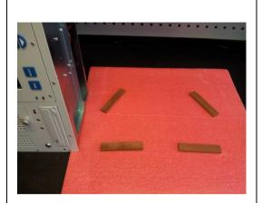
To remove the main face plate you must sit the unit at a small distance from the bench surface.
