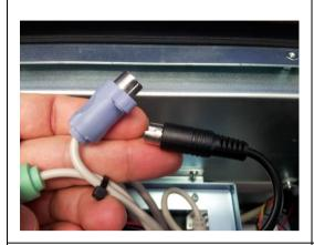
Identify the keyboard connector and connect the system keyboard to it.
