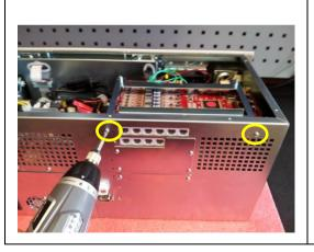
Remove the screws (2 in total) that hold the stack support frame.
