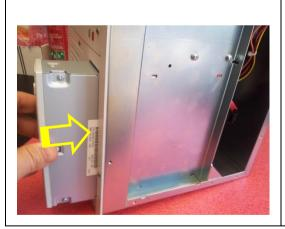
Insert the new disc drive into the enclosure.
