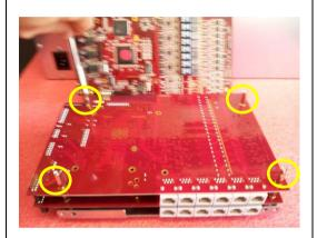
Attach the new card to the stack with 4 spacers.
