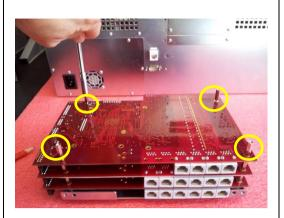
No add the card to the stack and attach it with the spacers.
