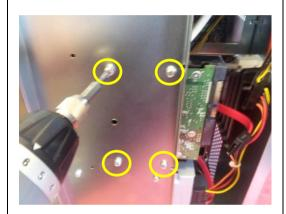
Remove the screws (4 in total) that bind the hard disk to the enclosure frame.
