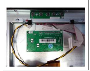
Place a new driver board in position on the frame.
