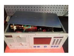
Finally, simply remove the top cover plate.
