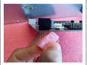
Remove the protective sponge from the power connector on the new card.
