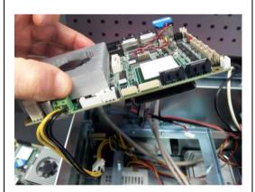
Carefully lift the SBC out of the enclosure.
