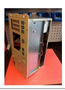
It is easier to replace the hard disk if you sit the unit on its side.
