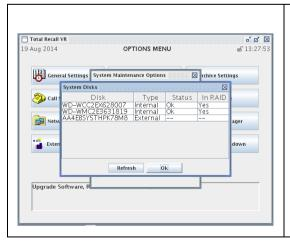
If you are hot replacing a drive then use the GUI application to detach the faulty drive from the system.
