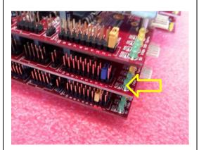
One final check of the jumpers on the J5 connectors. They need to be in position 1, 2, and 3 starting from the top card and moving towards the bottom card.
