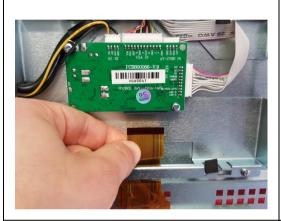
Pass the TTL cable of the replacement panel through the bottom hole of the panel frame.
