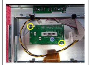
Detach the driver board from the frame. Remove 2 screws.
