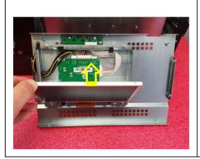
Lift the LCD panel and place it its frame.
