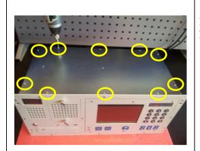
Fit the rest of the screws (10 in total) that hold the top cover plate in place.
