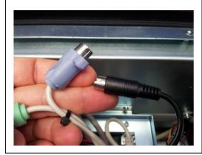
Remove the duct tape and disconnect the keyboard from the SBC.
