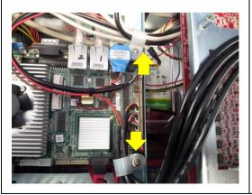
Replace the P clips (2 in total) that attach cables to the edges of the SBC.
