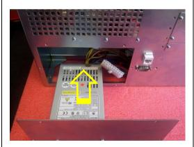
Insert the power supply into the enclosure.
