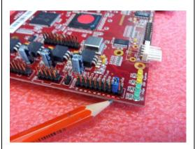
We will place the new card in position 2 in the stack (2<sup>nd</sup> card in the stack).
