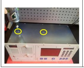
Remove the two screws that hold the stack of analogue channel cards first.
