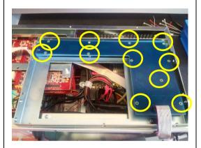
Replace the screws (11 in total) that bind the keyboard to the enclosure.
