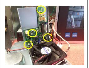
Remove the screws (4 in total) that bind the mid-board to the metal part.
