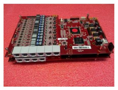
When stacking cards it is important to get two things right. First, the power connector, J10, must be connected correctly. Second, the stack position jumper, J5, must be set to the correct position: 1 for the first card, 2 for the second, 3 for the thirds card and so on.
