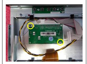
Attach the driver board to the frame. Replace 2 screws.
