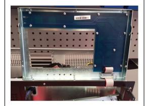
It should be possible to sit the keyboard assembly on the top edge of the unit.
