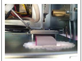
Another clamp holds the keyboard cable on the inside wall of the enclosure.
