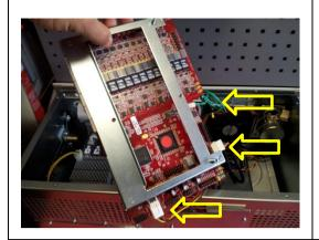
Lift the whole stack out of the enclosure.
