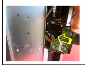
Insert the new hard disk into the enclosure.
