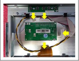
Disconnect the all cables from the VGA driver board.
