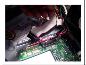
Start disconnecting cables from the midboard to free the assembly from the enclosure.
