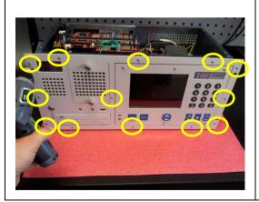
Remove the screws (13 in total) that hold the face plate in place.
