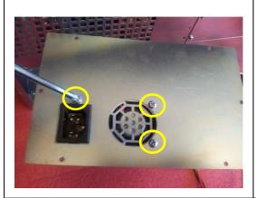
Fit the cover plate to the new power supply.
