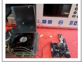
Finally, simply separate the mid-board from the sub-assembly.
