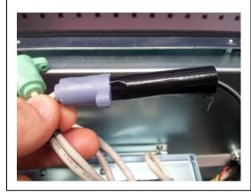
Replace the duct tape that stops the keyboard connectors from disconnecting.
