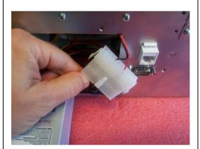
Attach the on/off key switch to the power supply.
