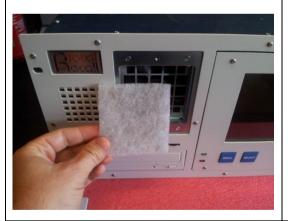
Then simply replace the filter with a new one.
