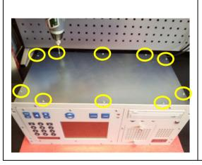
Fit the screws (10 in total) that hold the bottom cover plate in place.
