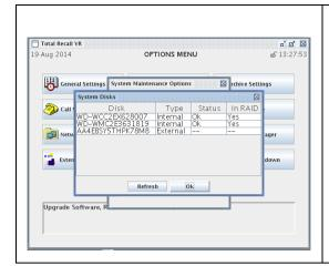
If you are hot replacing a drive then use the GUI application to attach the new drive to the system.
