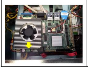
Disconnect all cables from the SBC except for the power cable (the arrow points to this cable).
