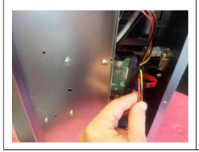
Attach the SATA and power cables to the hard disk.
