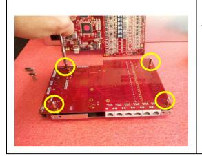
Attach it to the stack with the spacers.
