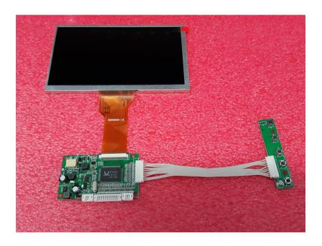
However, some Total Recall VR systems were fitted with a 6.4" LCD panel with LVDS interface. Inverters were used with such panels in order to power their back light.
