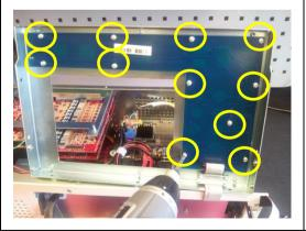
Remove the screws (11 in total) that bind the keyboard to the enclosure.
