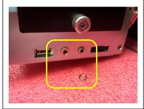
Remove the nuts from the two audio jacks.
