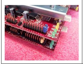
One final check of the jumpers on the J5 connectors. They need to be in position 1 and 2 starting from the top card and moving towards the bottom card.
