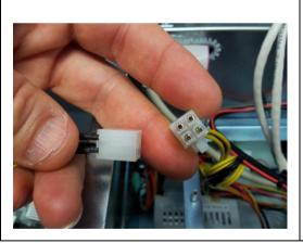
Attach the power cable from the SBC to the power supply.
