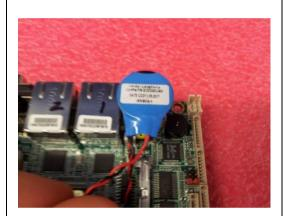
Attach the battery to the top of the USB port stack on the new SBC.
