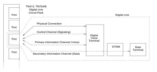
Figure 5-19. Digital Line Connectivity
