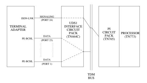
Figure 5-48. PRI Endpoint Port Interactions [INTEL]
