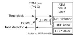
Figure 5-11. ATM Board DSP Test (#1293)
