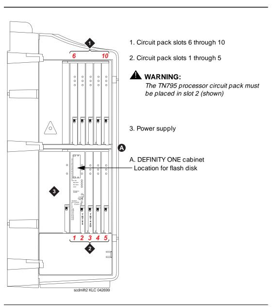
Figure 1-1. Compact Modular Cabinet (CMC) slot configuration
