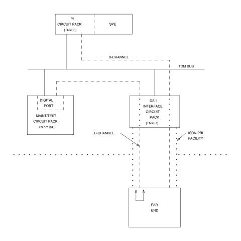
Figure 5-44. ISDN-PRI Outgoing Test Call
