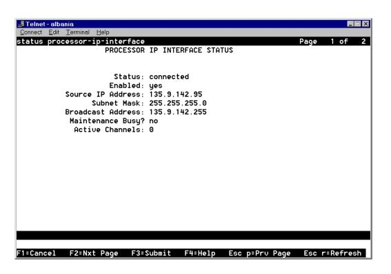
Figure 1-8. Processor interface status
