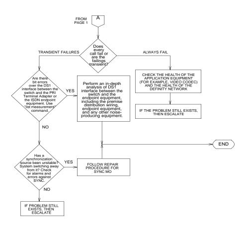
Figure 2-9. Processing of PRI endpoint problems (page 2 of 2)
