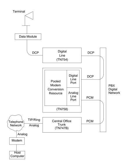
Figure 5-40. Typical Modem Pool Switched Connection with Integrated Pooled Modem
