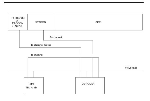
Figure 5-30. ISDN-PRI Outgoing Test Call
