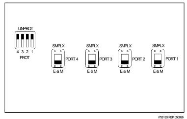
Figure 2-17. TN760D tie trunk circuit pack (component side)
