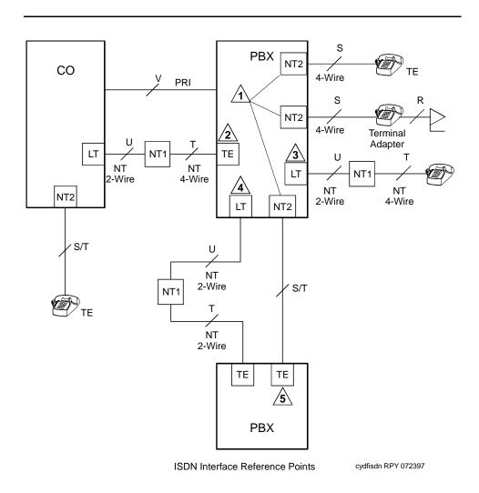
Figure 5-52. Integrated Trunk-Side BRI, ISDN Interface Reference Points
