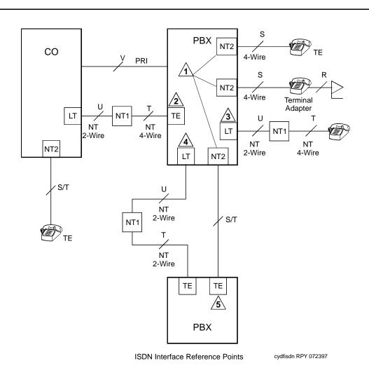
Figure 5-53. Integrated Trunk-Side BRI, ISDN Interface Reference points
