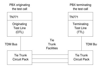
Figure 5-43. ATMS Tie Trunk Test Call
