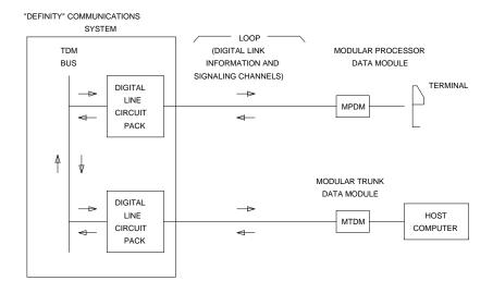
Figure 5-46. Typical Data Module Application
