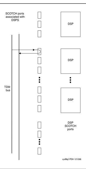
Figure 5-59. VC Circuit Pack DSP Port Local TDM Loopback Test
