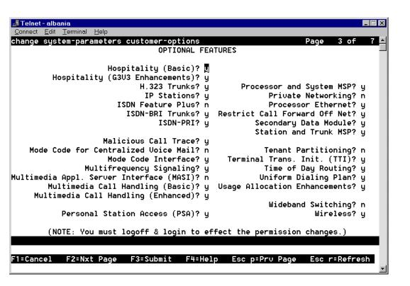
Figure 1-7. Processor ethernet customer option entry
