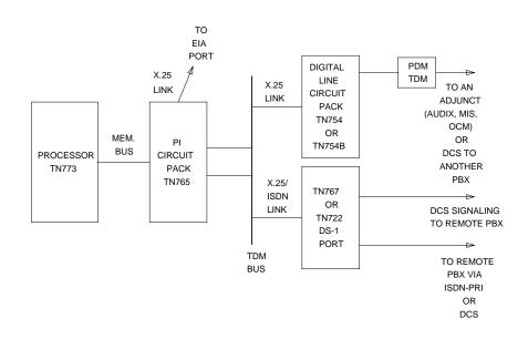
Figure 5-50. Processor Interface Link Interactions
