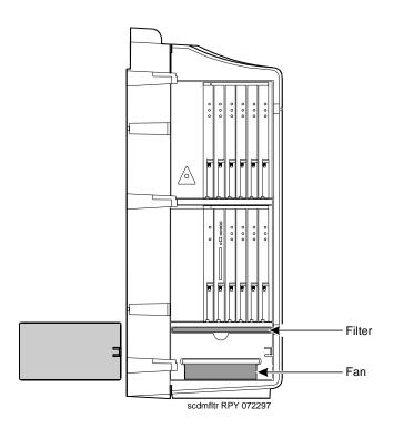
Figure 2-1. Fan/filter removal
