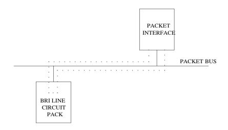
Figure 5-13. Path of the BRI Port Local LAN Loop Around
