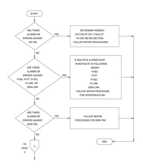
Figure 2-6. Processing of ISDN-PRI problems (page 1 of 2)
