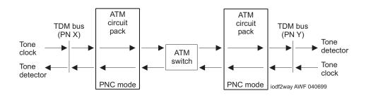
Figure 5-6. Expansion Interface 2-Way Transmit Test #241 PN X and PN Y represent any of 43 possible port networks.
