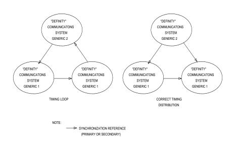
Figure 5-51. Synchronization Timing Loop
