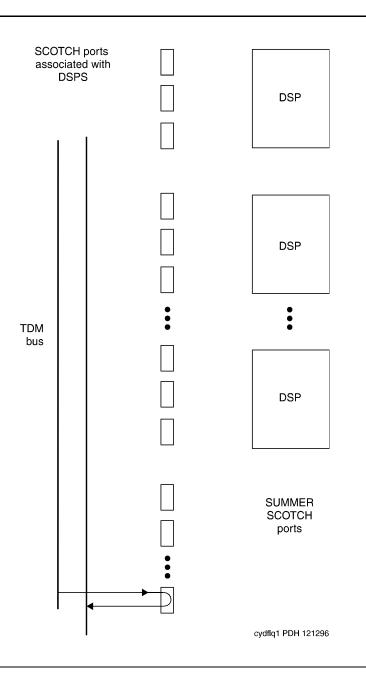
Figure 5-61. VC Circuit Pack Summer Port Loopback Test
