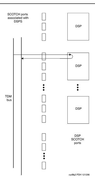
Figure 5-60. VC Circuit pack DSP Port DSP Looparound Test
