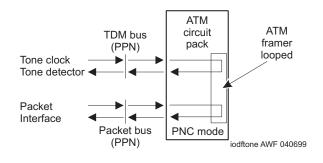
Figure 5-8. ATM Board Framer Looparound Test (#1260)
