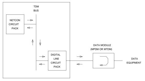
Figure 5-47. Internal Loop Around Test
