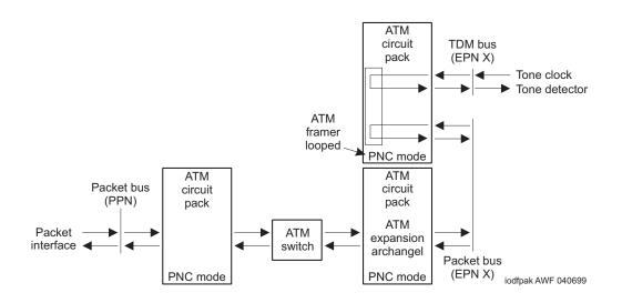
Figure 5-9. ATM Board Framer Looparound Test (#1260) (non-EAA, Packet Path)
