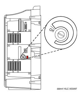
Figure 2-2. Setting the neon voltage
