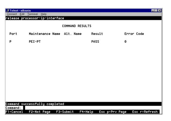
Figure 1-6. DLG release-from-busyout results
